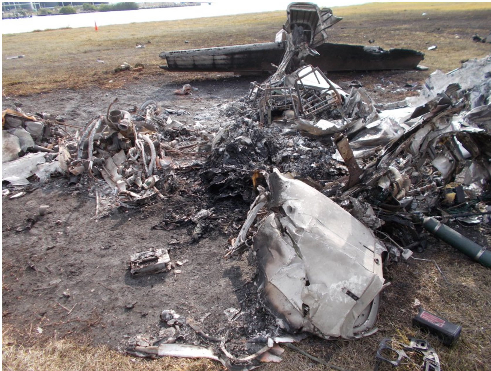
Photo 6 - NTSB Digital Photograph. View of the Cessna 340A Aircraft Nose Section, Portion of Instrument Panel, Separated Instruments, and Cabin in Background. Note the Extensive Fire Damage.
