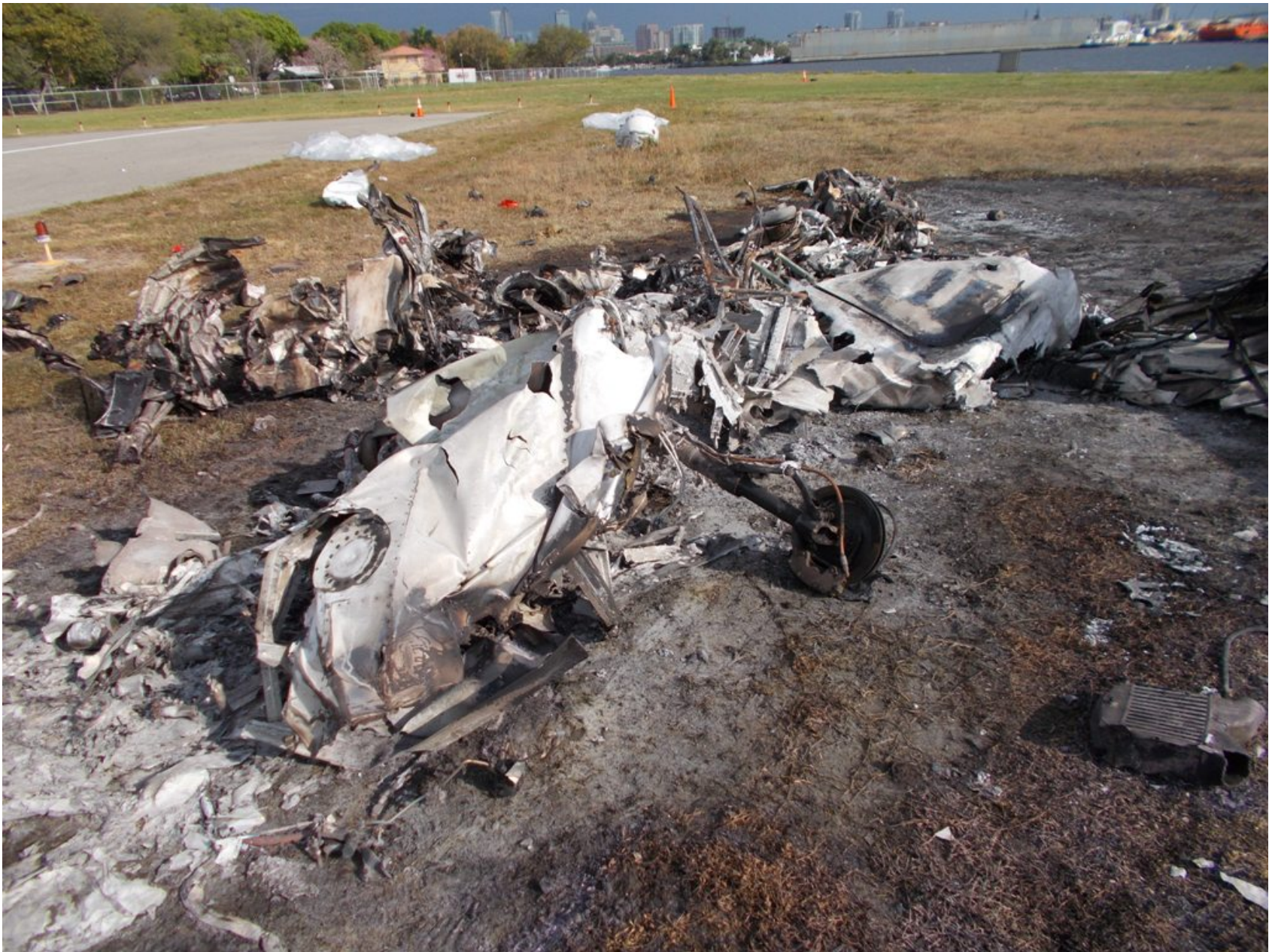
Photo 5 - NTSB Digital Photograph. Close-Up View of the Cessna 340A Main Wreckage. Note the Extensive Fire Damage.
