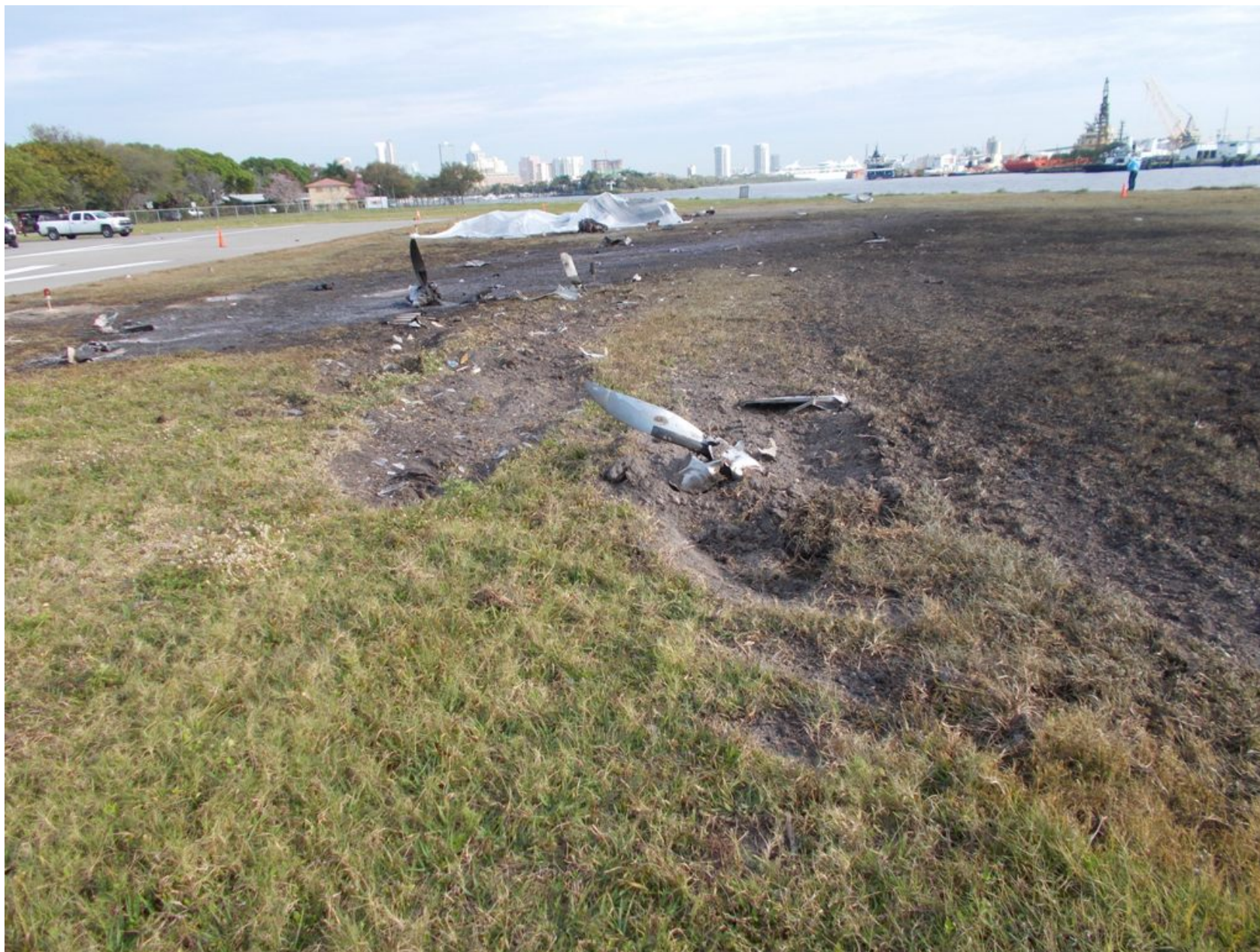
Photo 2 - NTSB Digital Photograph. View of the Cessna 340A Initial Impact Site. Note the Separated Propellers and ground scars from the left propeller and upper portion of the forward fuselage.
