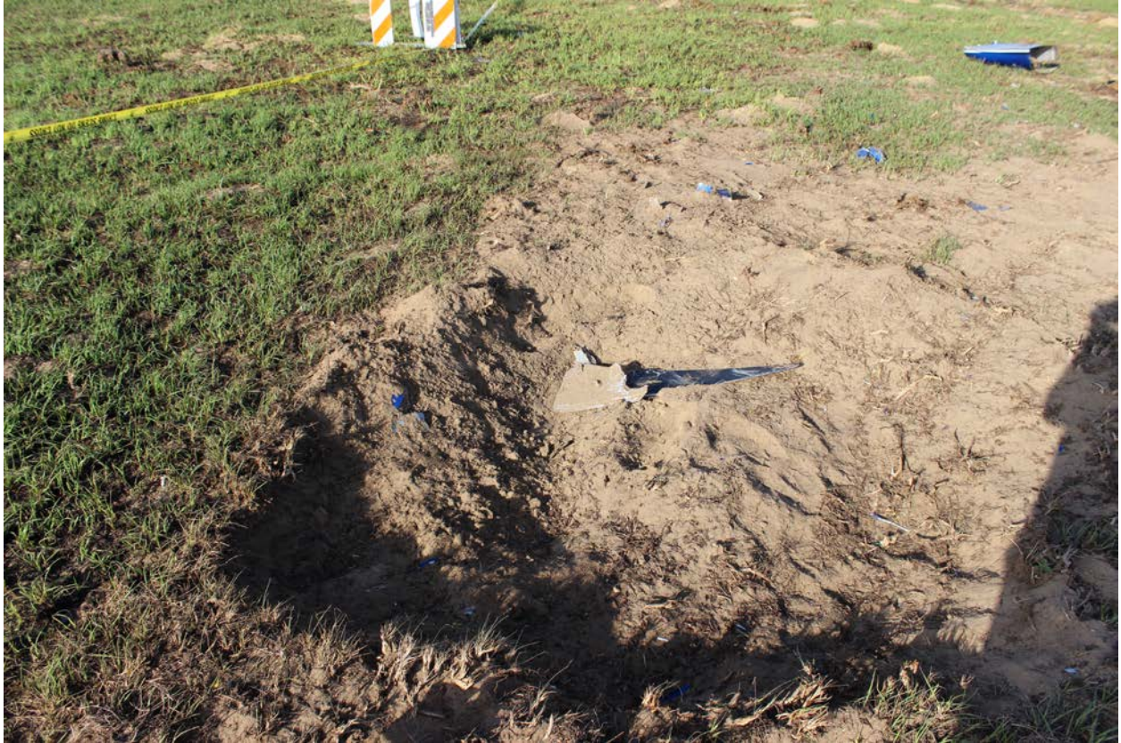
Figure 3 Impact crater with a portion of a propeller blade.
