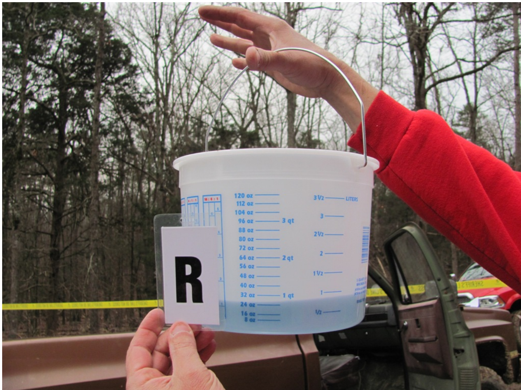
Photo 5 – Fuel Drained from Right Tank
