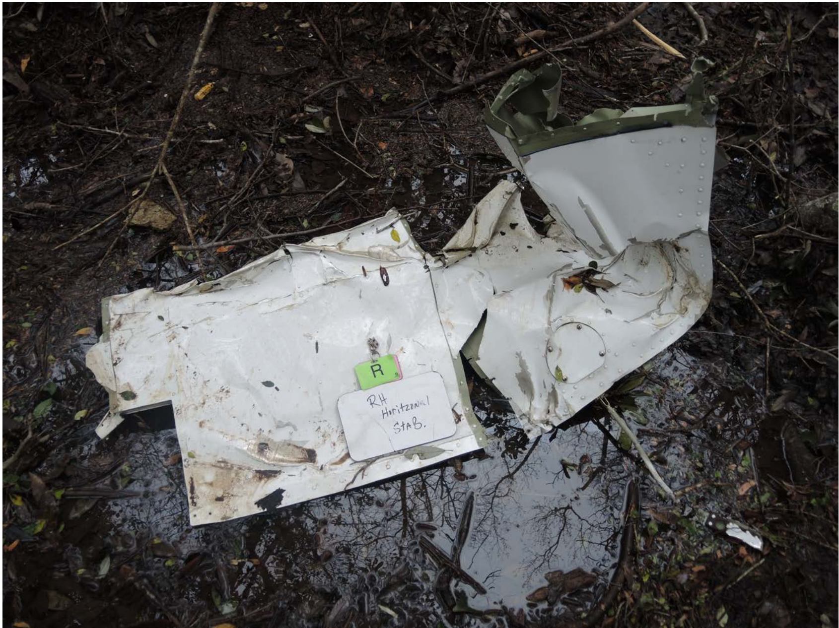
Photo 7 – View of damaged right horizontal stabilizer
