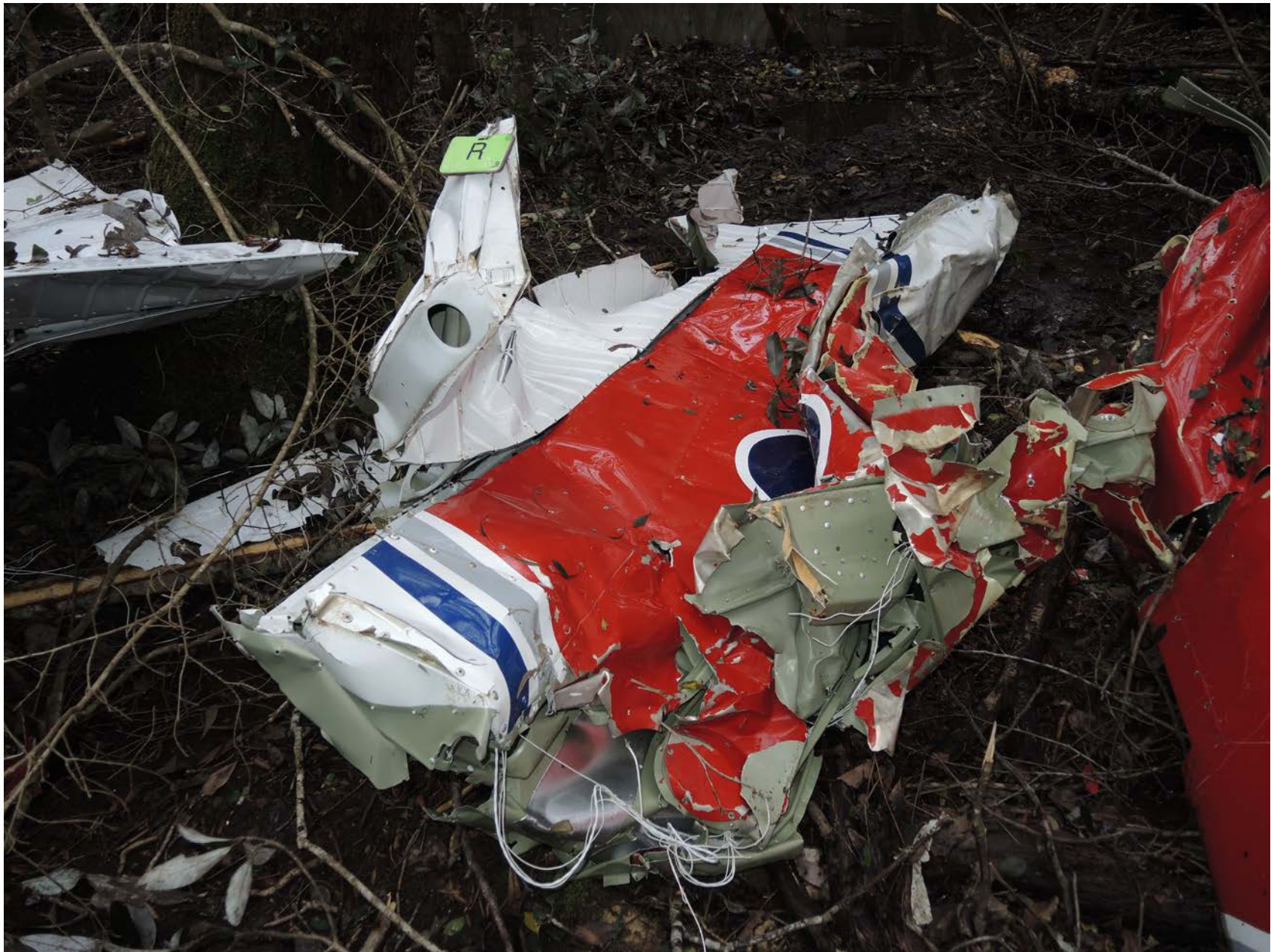
Photo 4 - View of damaged inboard right wing
