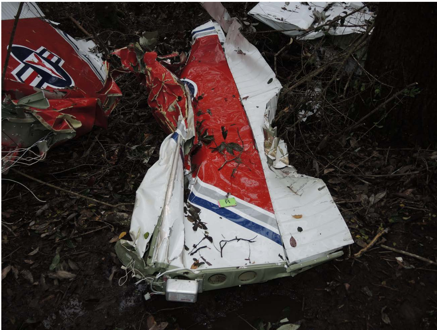
Photo 3 – View of damaged outboard right wing
