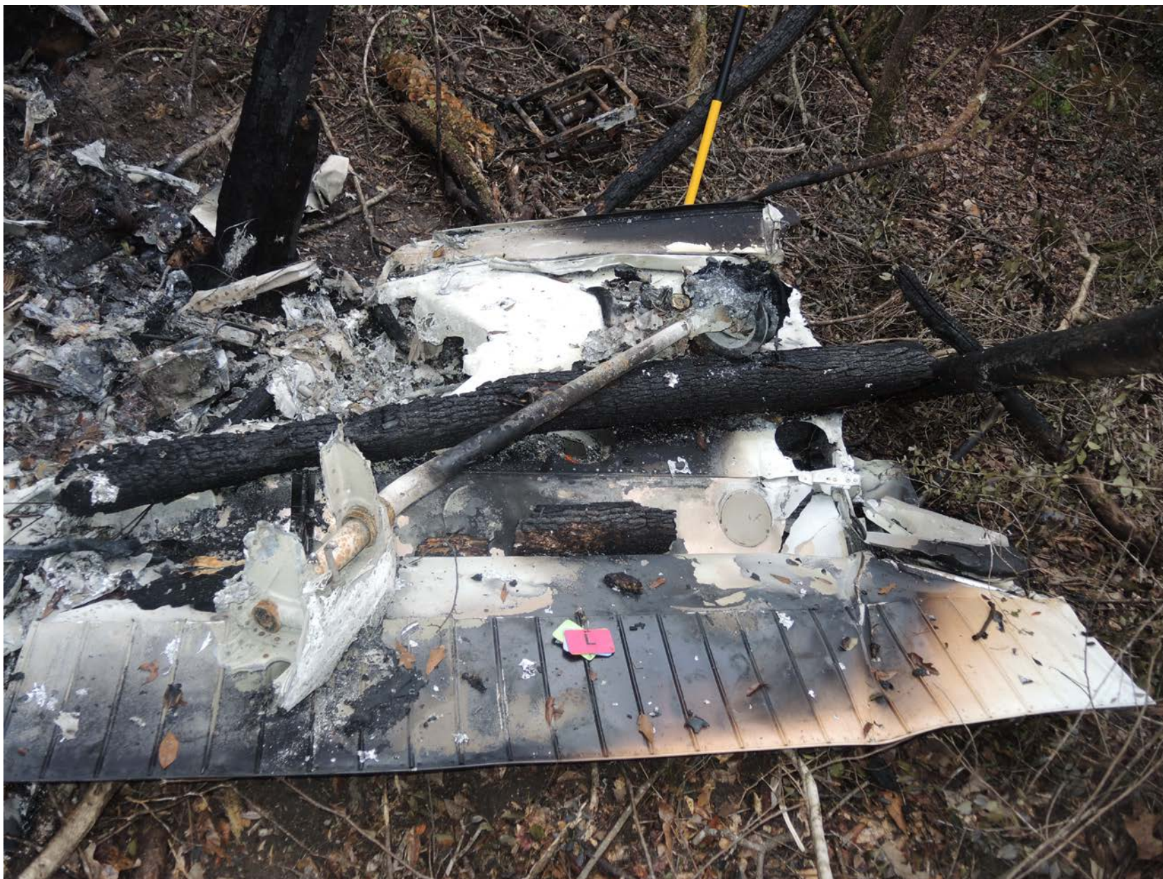
Photo 10 – View of fire damaged inboard left wing
