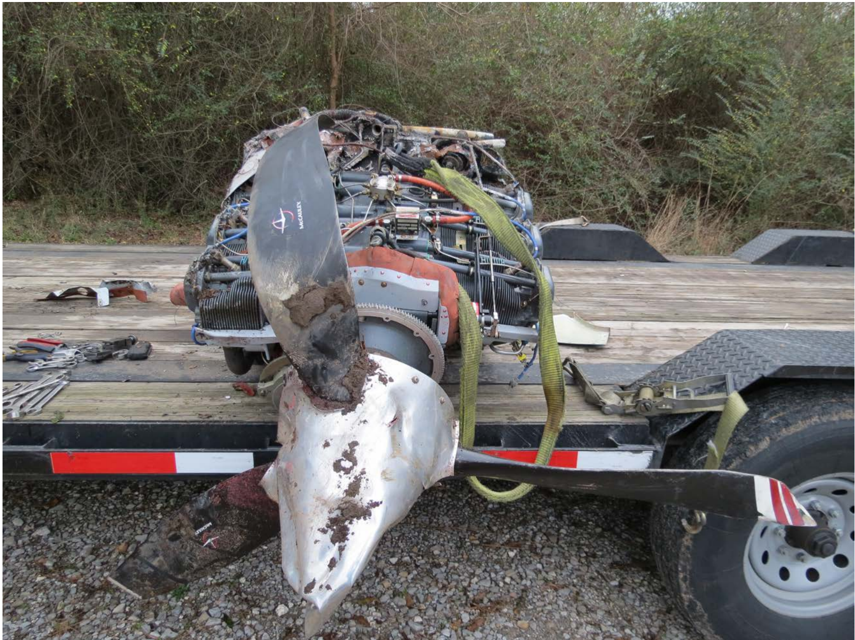
Photo 12 – Front view of damaged engine
