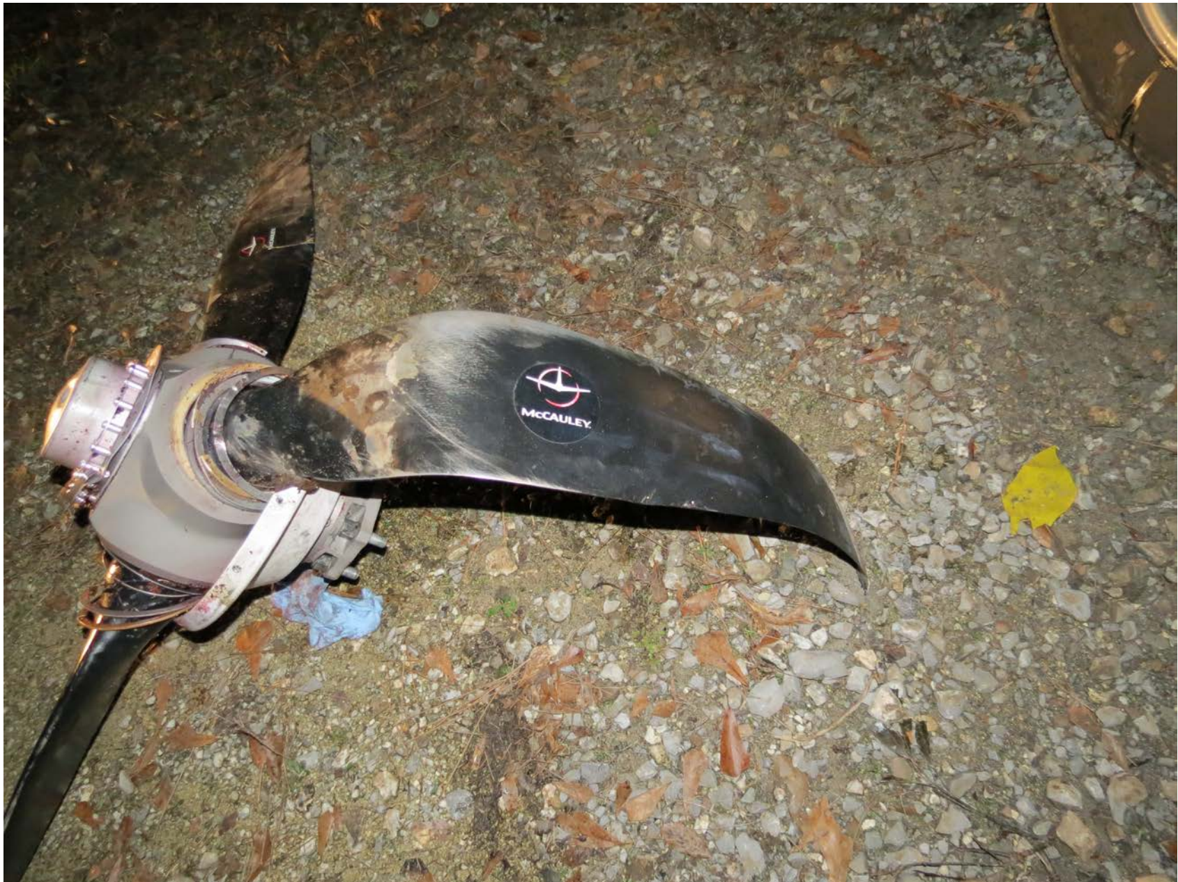
Photo 18 - Top view of propeller showing damaged blades
