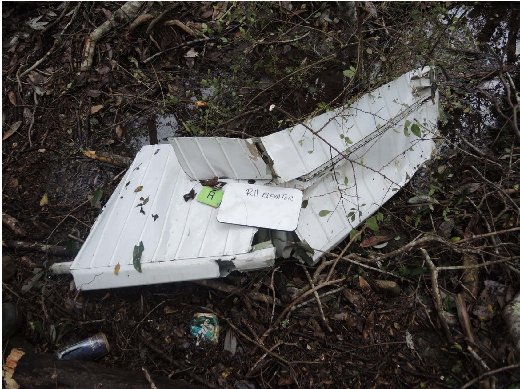
Photo 6 – View of damaged right elevator
