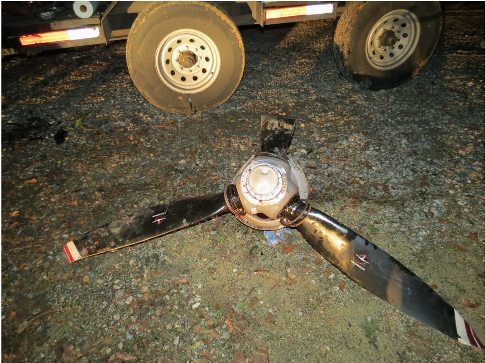
Photo 17 – Front view of propeller showing damaged blades
