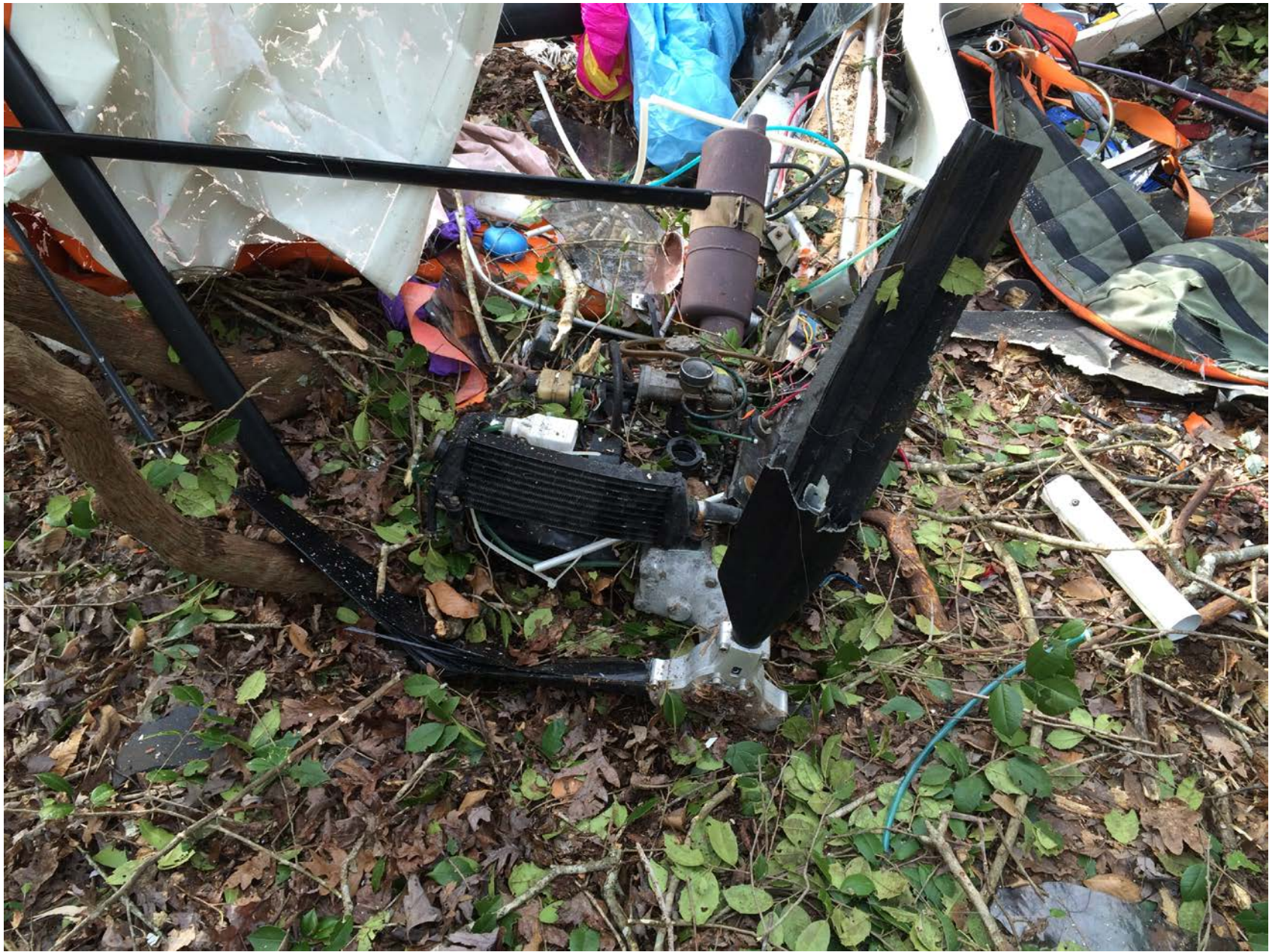
Photo 4 – Engine and Propeller Damage
