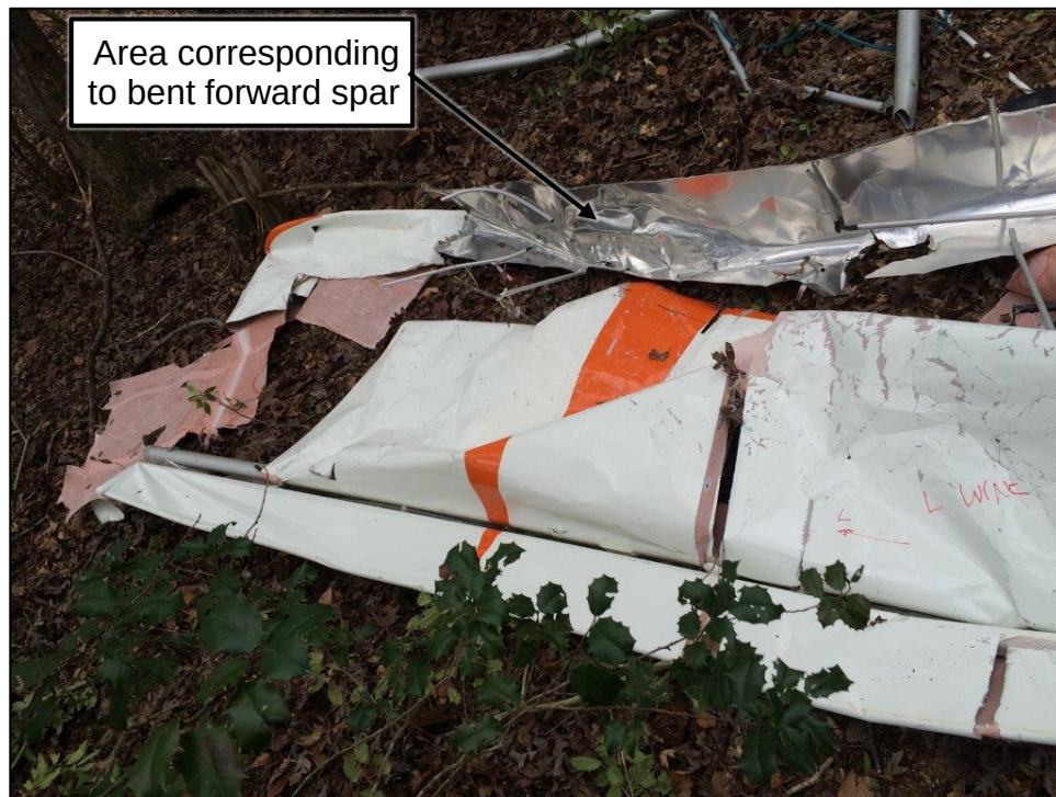
Figure 3. Left wing skin and leading edge strip as viewed on-scene.
