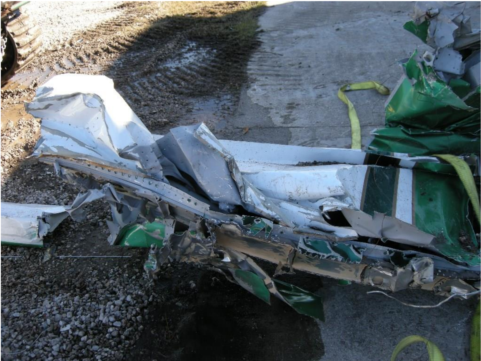
Photo 9 – Right Wing (NTSB Photo)
