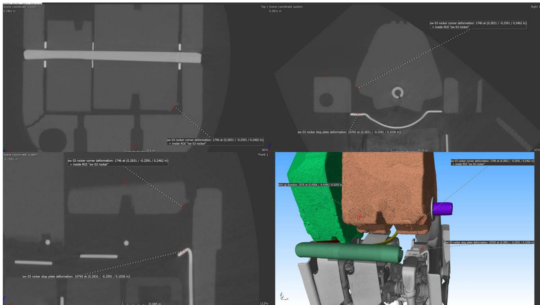
Figure 51 Autopilot trim switch assembly – Switch 03 (sw 03) rocker corner and stop plate deformation
