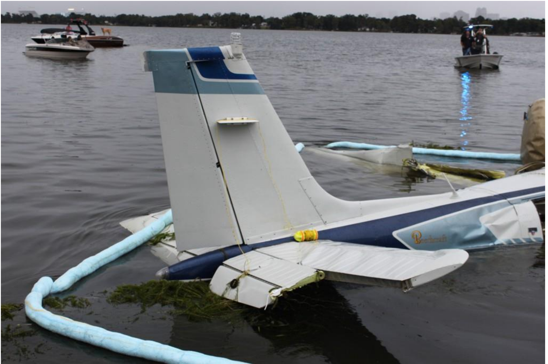
Photo 4 - NTSB Digital Photograph. View of the Right Side of the Empennage Before Recovery from the Water. Note the Position of the Right Elevator Trim Tab
