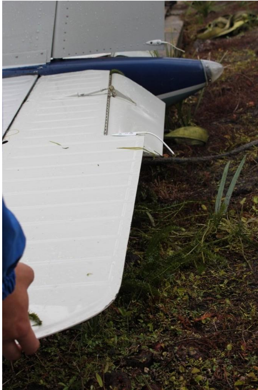
Photo 5 - NTSB Digital Photograph. Left Side View of the Left Elevator, Elevator Trim Tab, and Portions of Vertical and Horizontal Stabilizer and Rudder.
