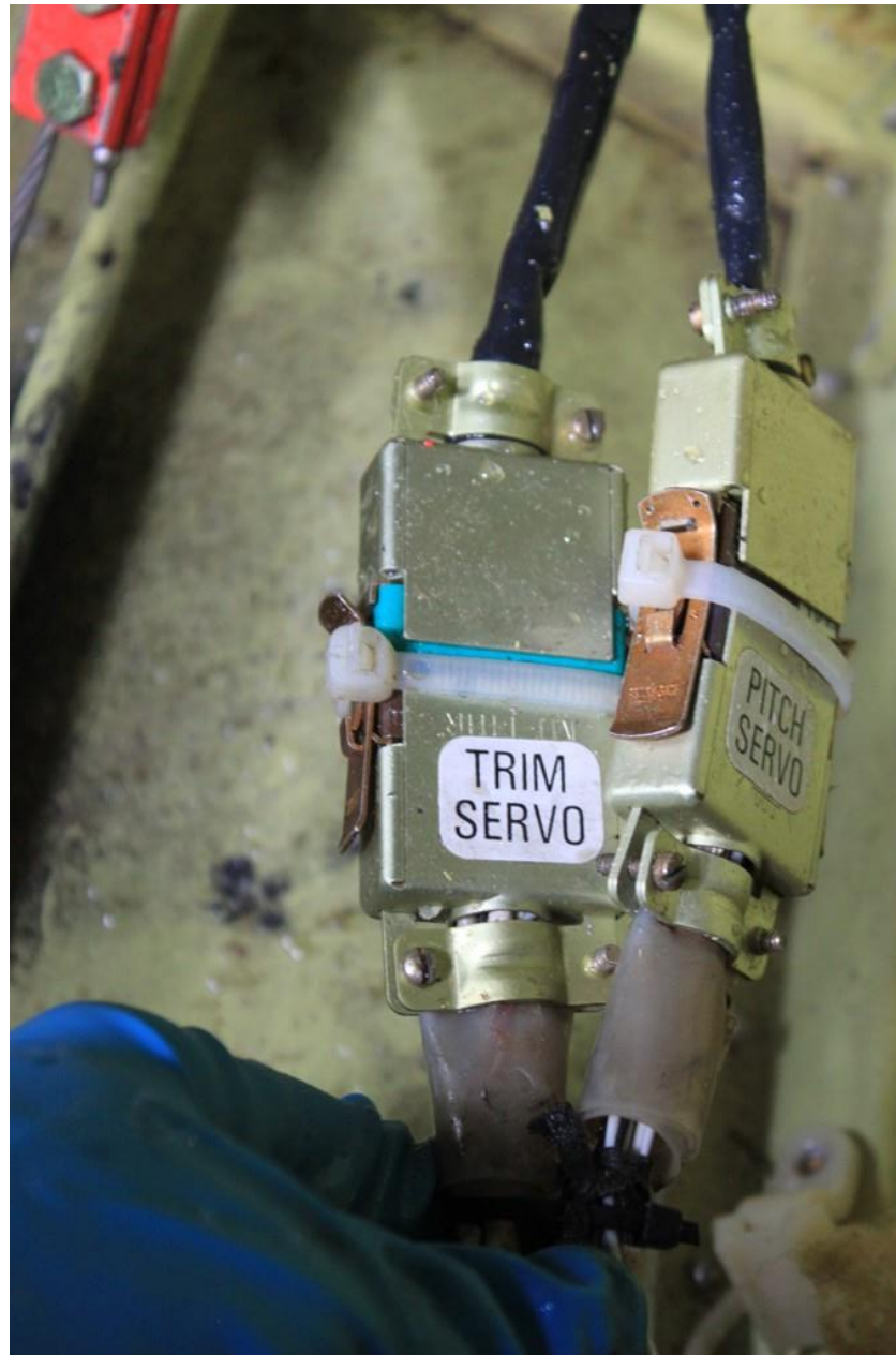
Photo 12 - NTSB Digital Photograph. View of the Connections for Trim and Pitch Trim Servos
