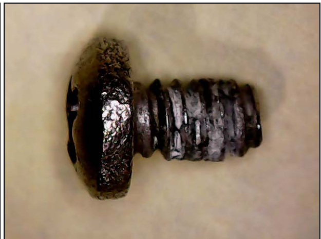
Screw securing circuit module assembly to the base plate assembly. Aluminum colored material in the threads.
