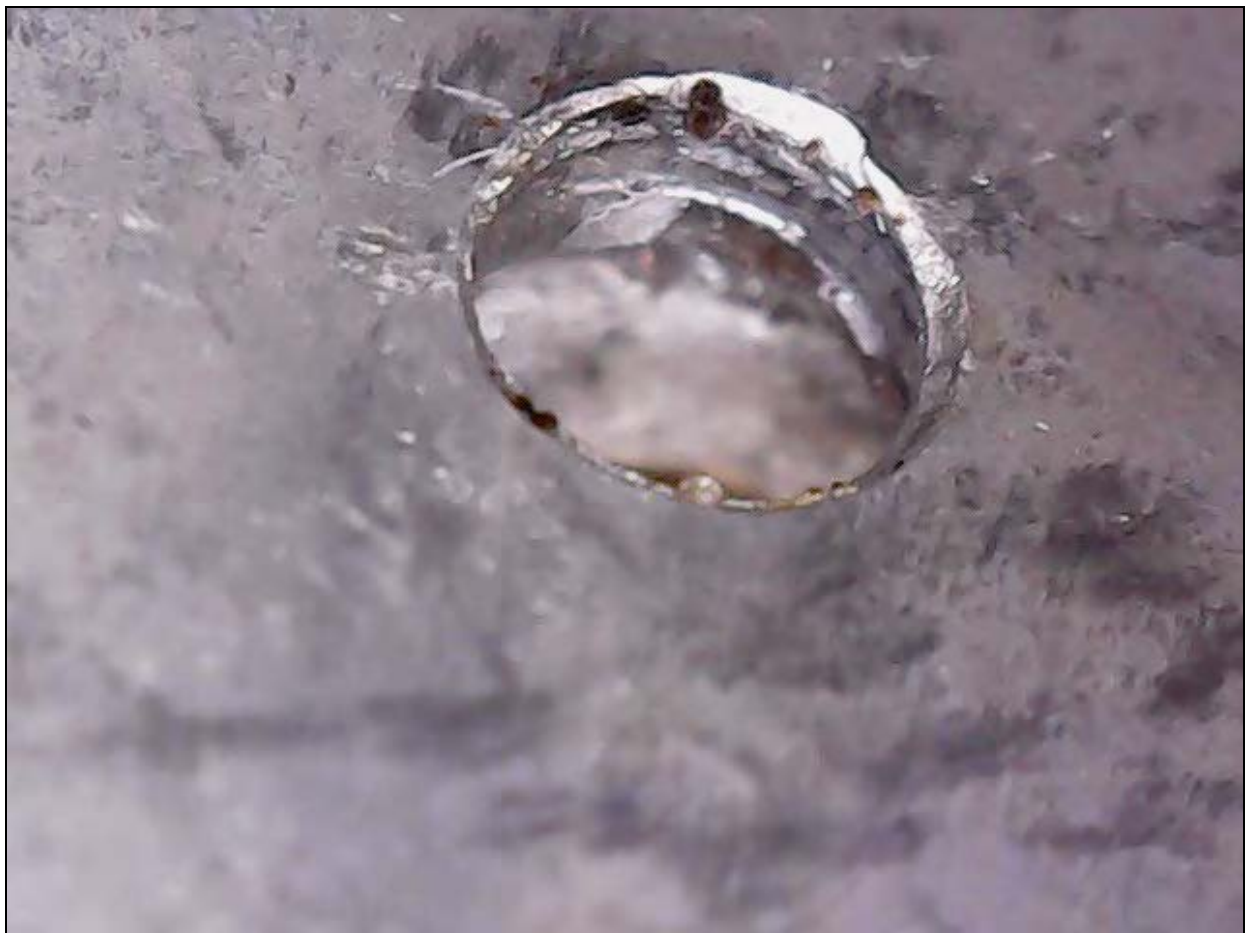
Screw hole in the servo baseplate – thread damage
