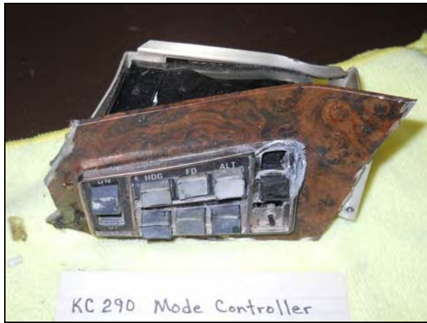
KC 290 Mode Controller is impact damaged which precludes functional testing
