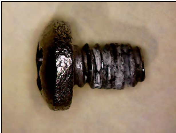
Screw securing circuit module assembly to the base plate assembly. Aluminum colored material located in the threads. The screw installs in the servo baseplate location shown in the following photo – notice damage or absence of threads.
