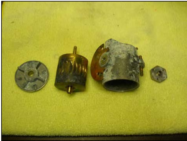
KI 256: rotor and capsule corroded
