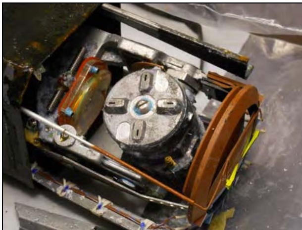
KI 256: removing the capsule and rotor assembly
