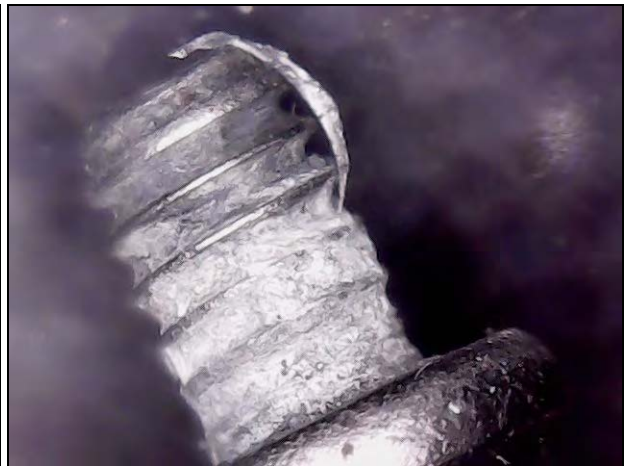
Screw securing circuit module assembly to the base plate assembly. Aluminum colored material located in the threads. The screw installs in the servo baseplate location shown in the following photo – notice damage or absence of threads.
