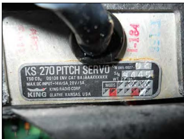
KS 270 Pitch Servo Dataplate: P/N 065-0027-02, S/N 9445
