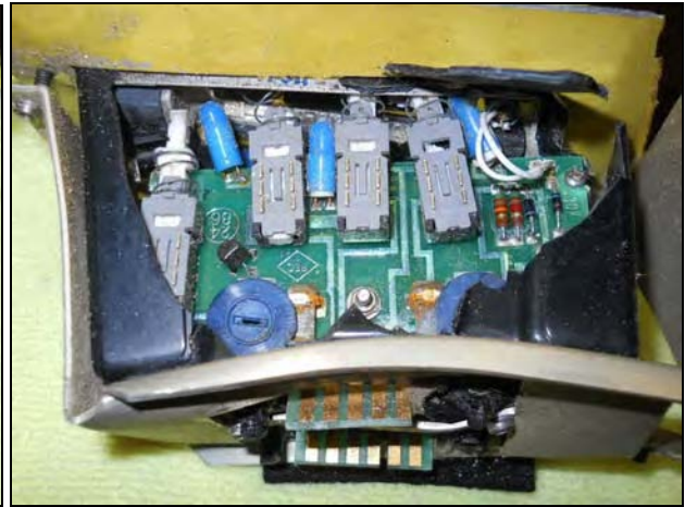
KC 290 Mode Controller is impact damaged which precludes functional testing
