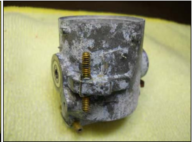
KI 256: rotor and capsule corroded
