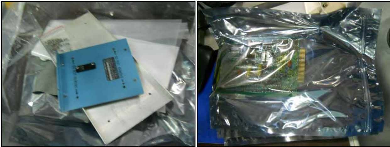
KC 295 Flight Computer as-received from the NTSB Lab – disassembled chassis on the left, circuit boards on the right
