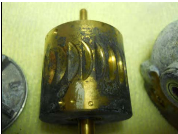
KI 256: no rotation scoring observed on the rotor or capsule
