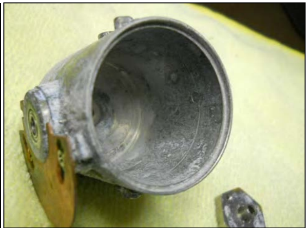
KI 256: no rotation scoring observed on the rotor or capsule
