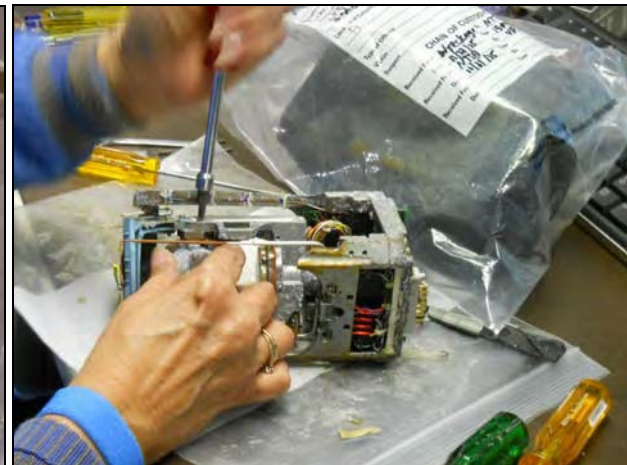
KI 256: removing the capsule and rotor assembly
