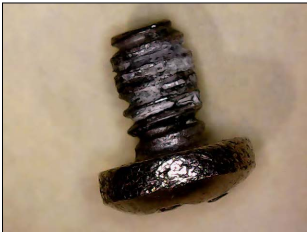
Screw securing circuit module assembly to the base plate assembly. Aluminum colored material in the threads.
