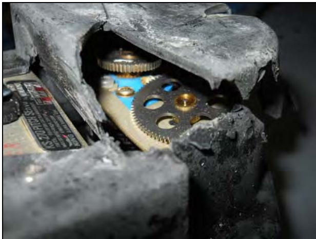
KS 270 Pitch Servo: internal damage – bracket bent, gears don't mesh
