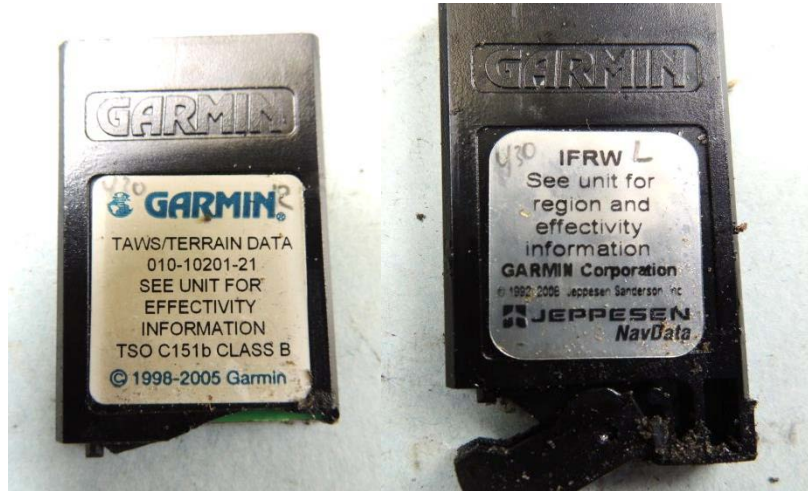
Figure 2. Database cards recovered from the Garmin GNS 530.
