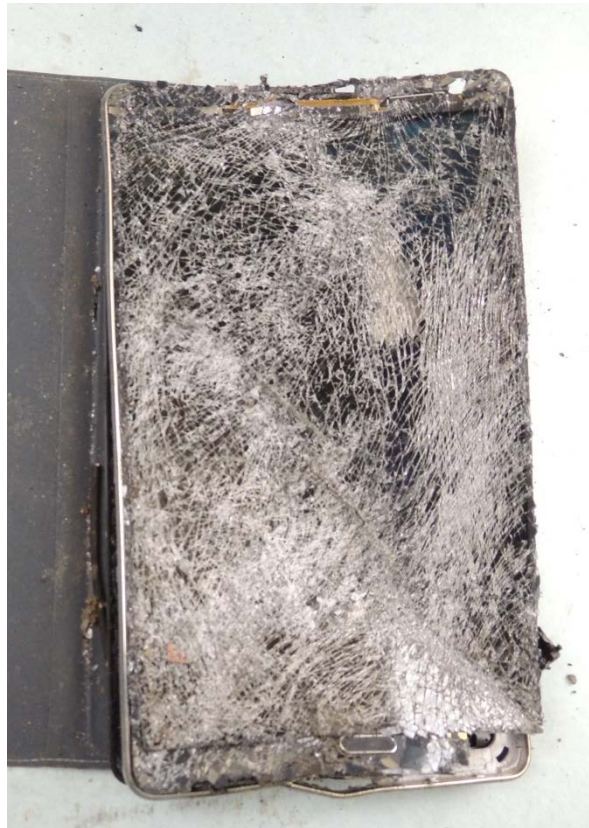
Figure 3. External view of the Samsung Galaxy Note II as received.
