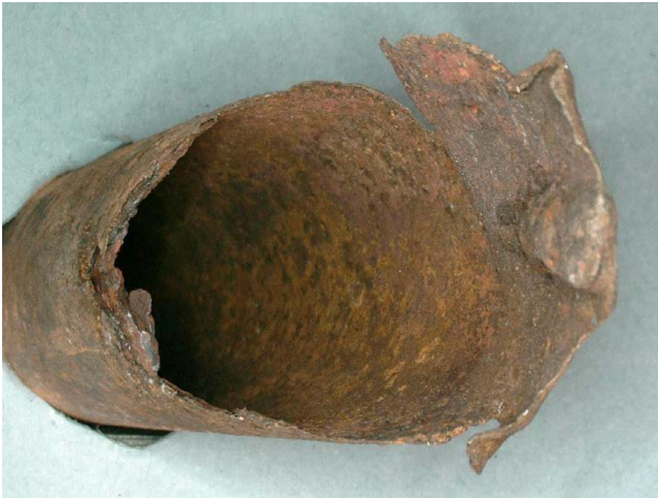
Figure 5. Two views of the left wing forward strut tube separation showing the severe corrosion thinning of the tube wall at the separation.
