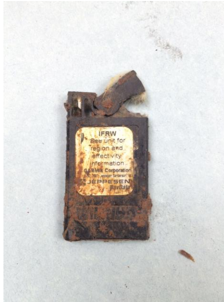
Figure 1. Damaged Garmin Database Card.
