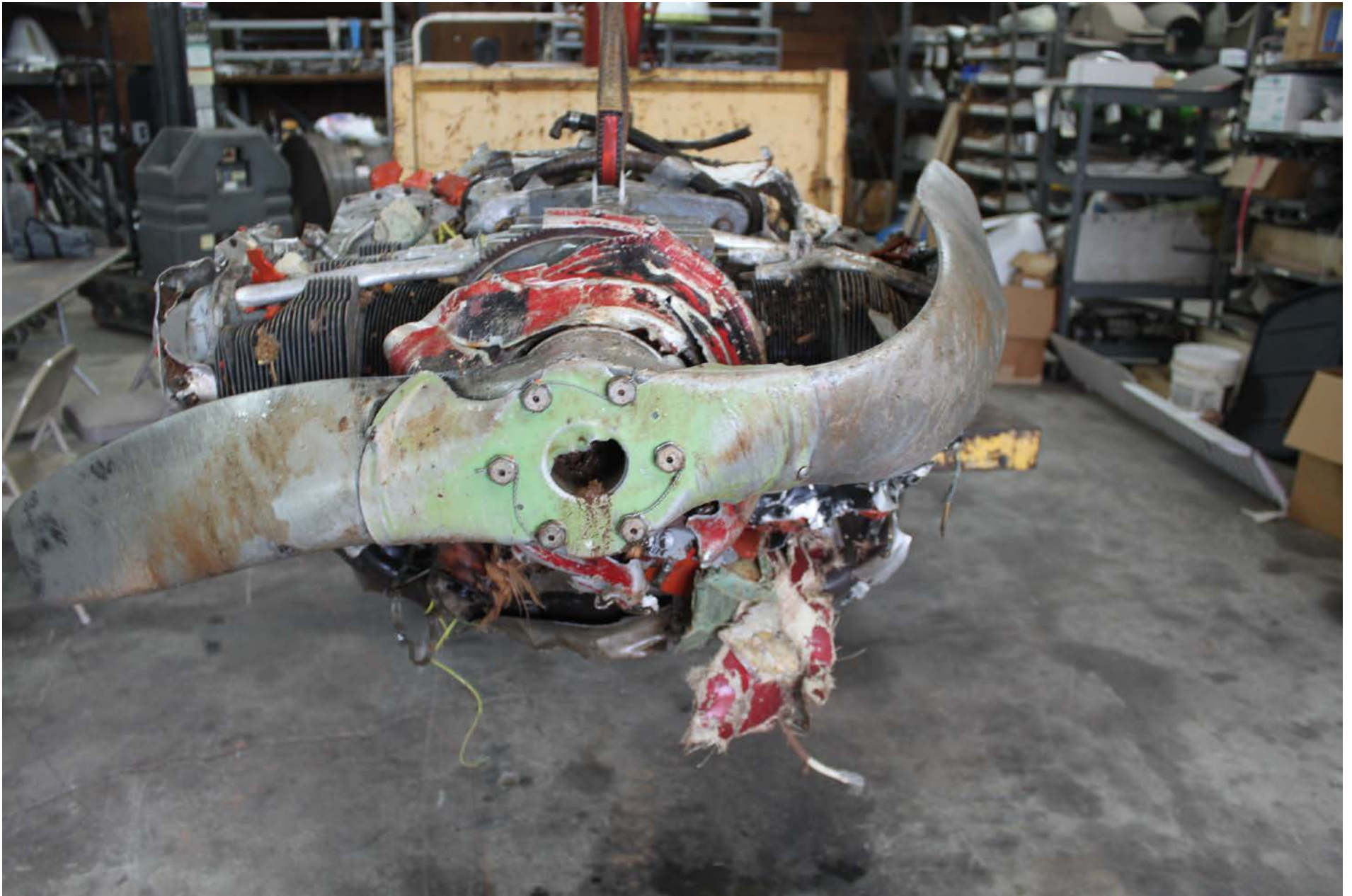
Photo 4 - View of front of engine and damaged propeller
