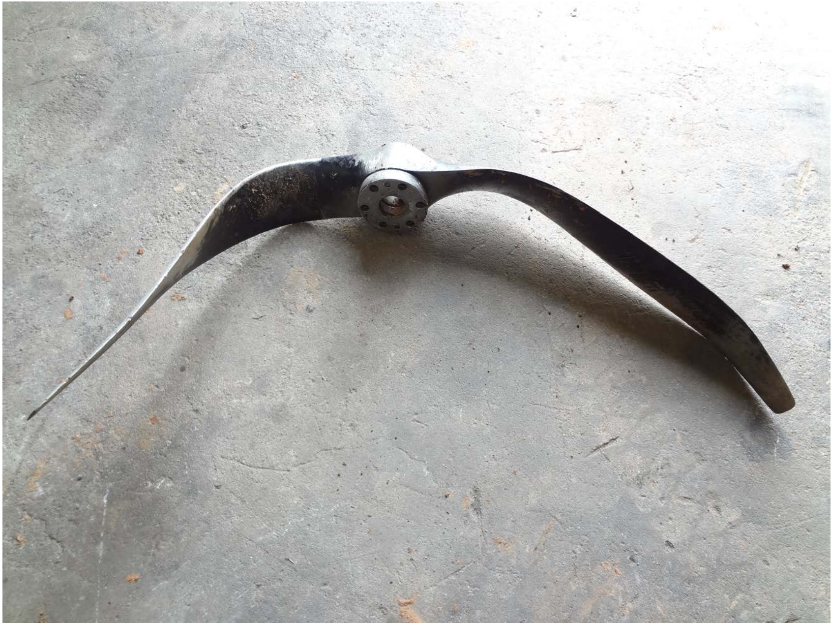
Photo 6 – View of propeller removed from flange showing twisting and bending
