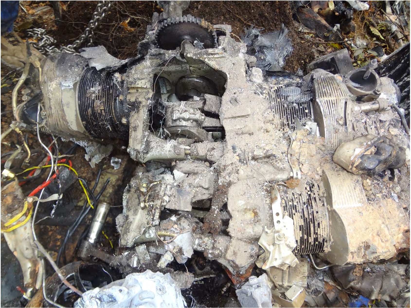
Photo 6 - Engine after Extraction from the Ground
