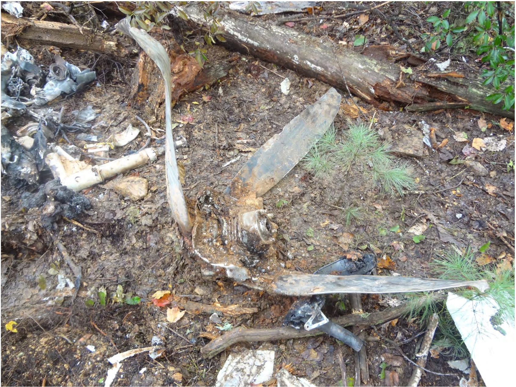
Photo 8 - Propeller Blades after Removal from the Impact Crater
