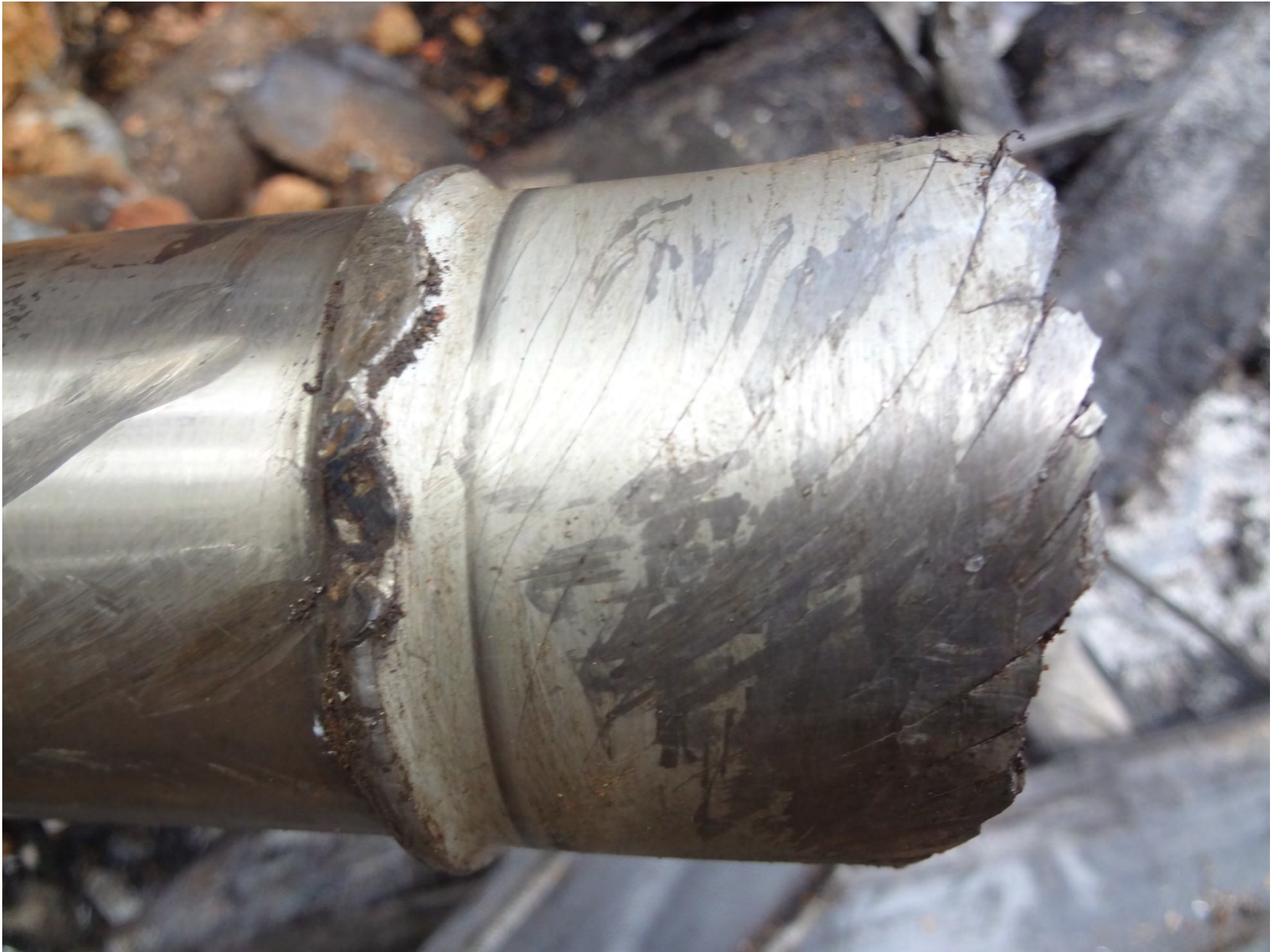
Photo 7 - Crankshaft Striation as found
