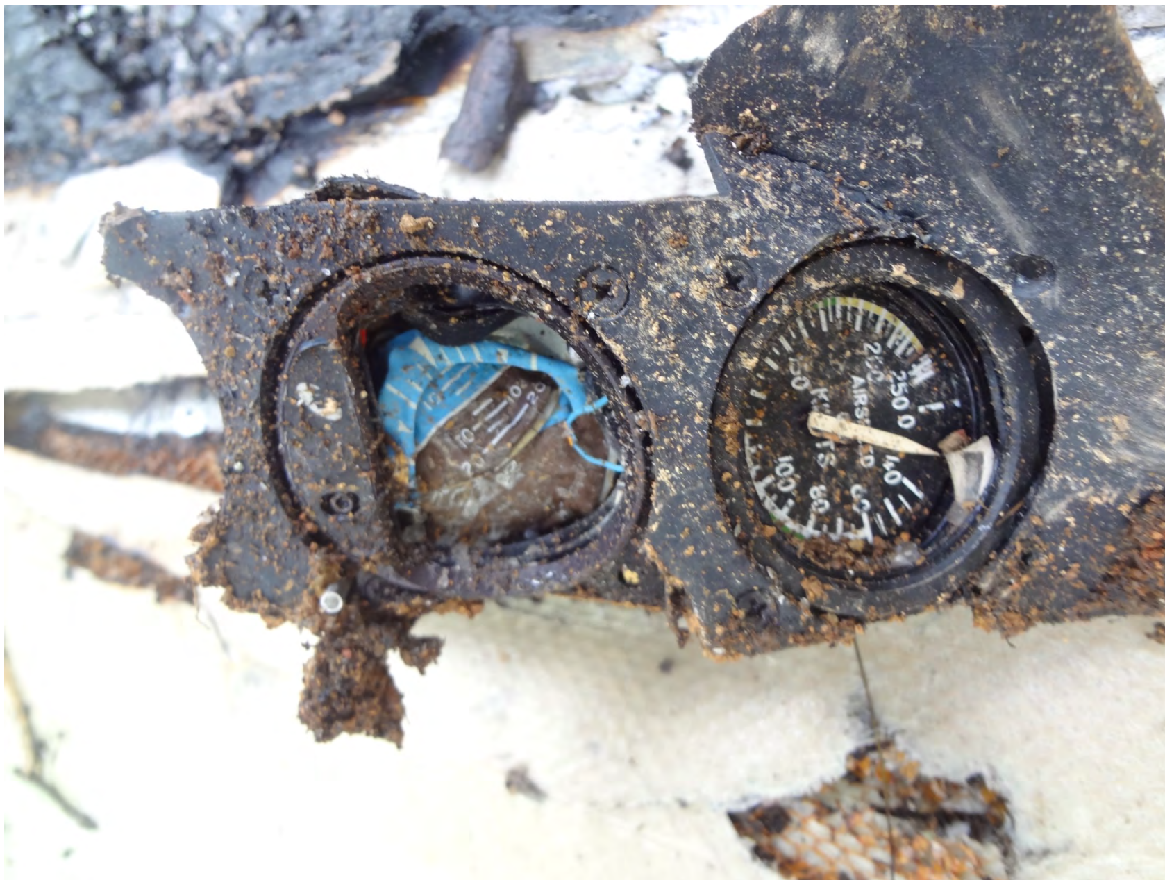
Photo 5 - Backup Attitude Indicator and Airspeed indicator as found
