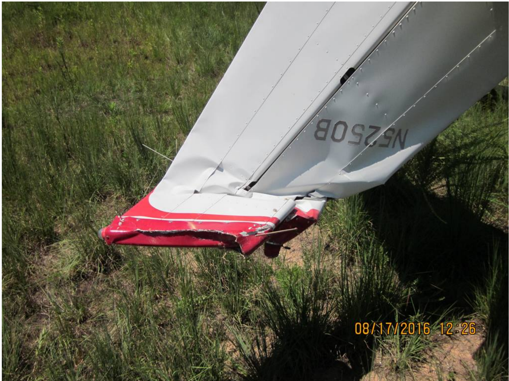
Photo 2 – Vertical Stabilizer and Rudder Damage
