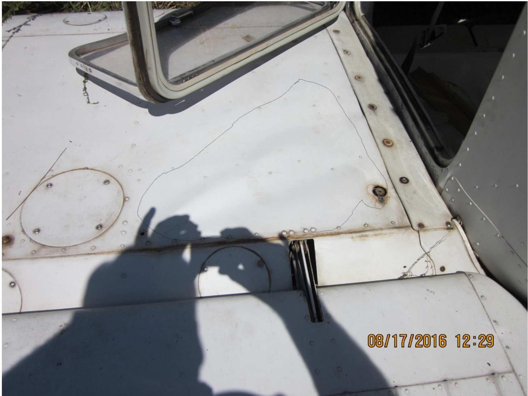
Photo 3 – Wing Buckling (FAA Photo)
