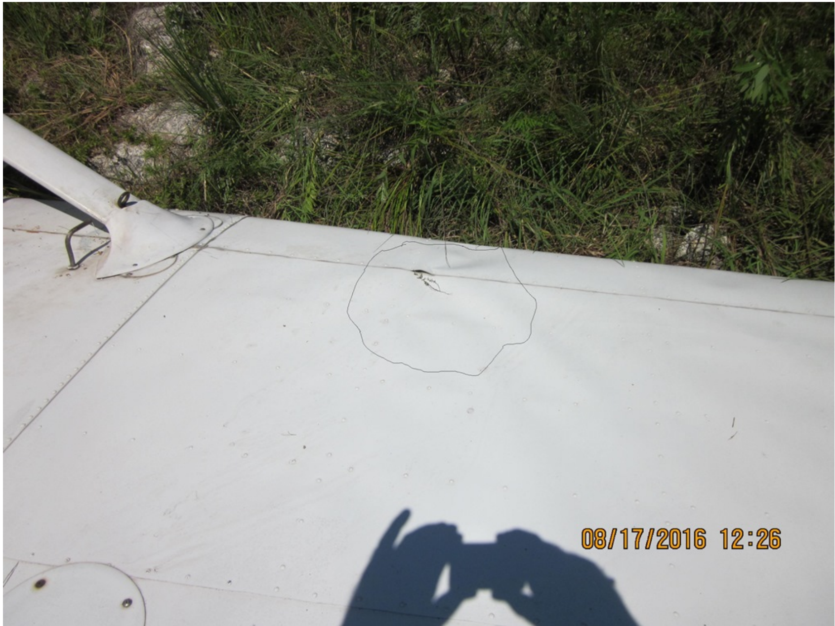
Photo 4 – Wing Buckling (FAA Photo)
