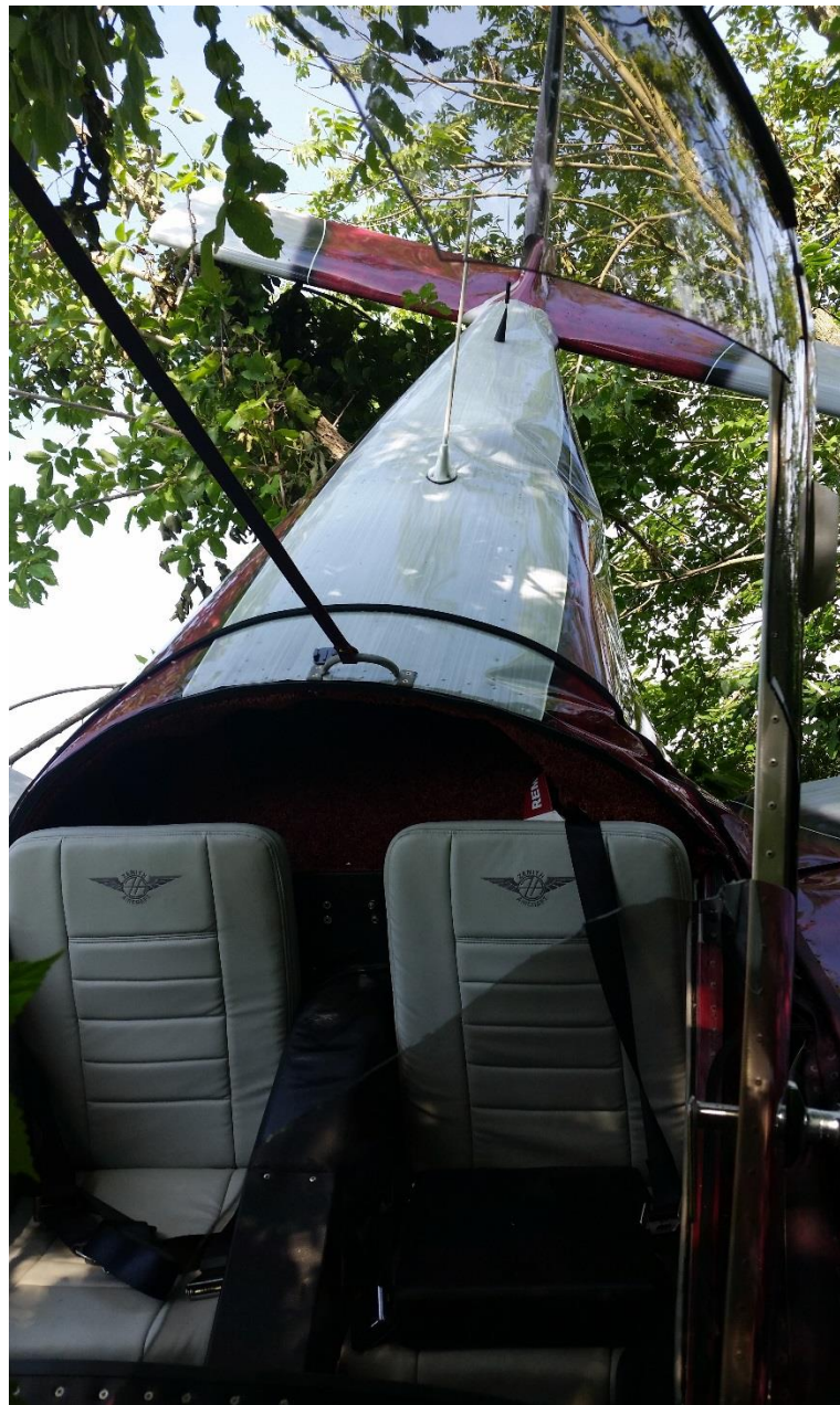
Photo 1 – Cockpit looking Aft Towards Tail; Tail Twisted to the Left (Courtesy of FAA)
