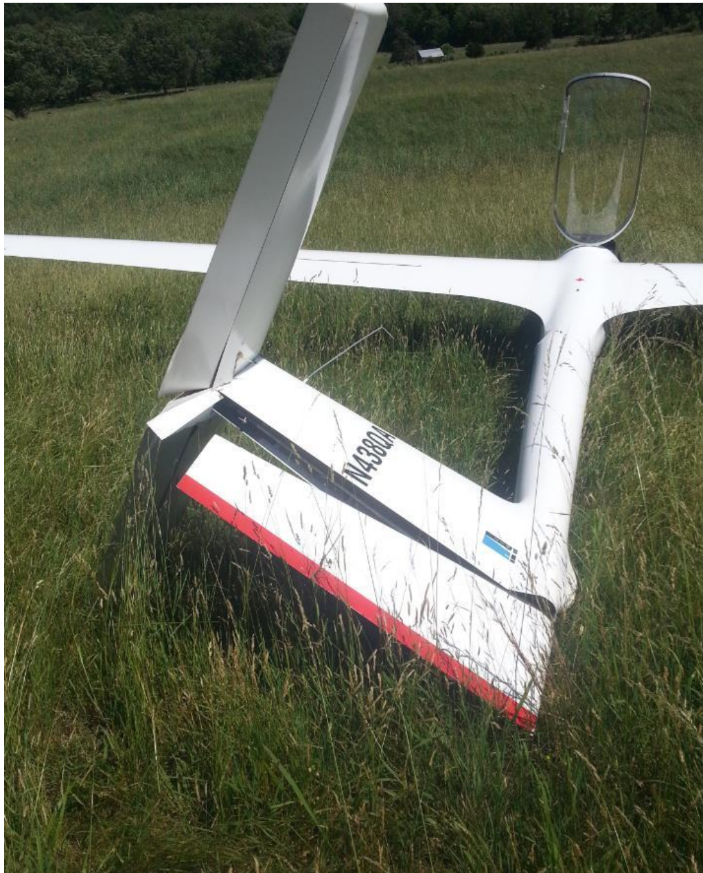
Photo 2 – Fuselage and Tail Damage; Tail Twisted to the Left (Courtesy of Pilot)
