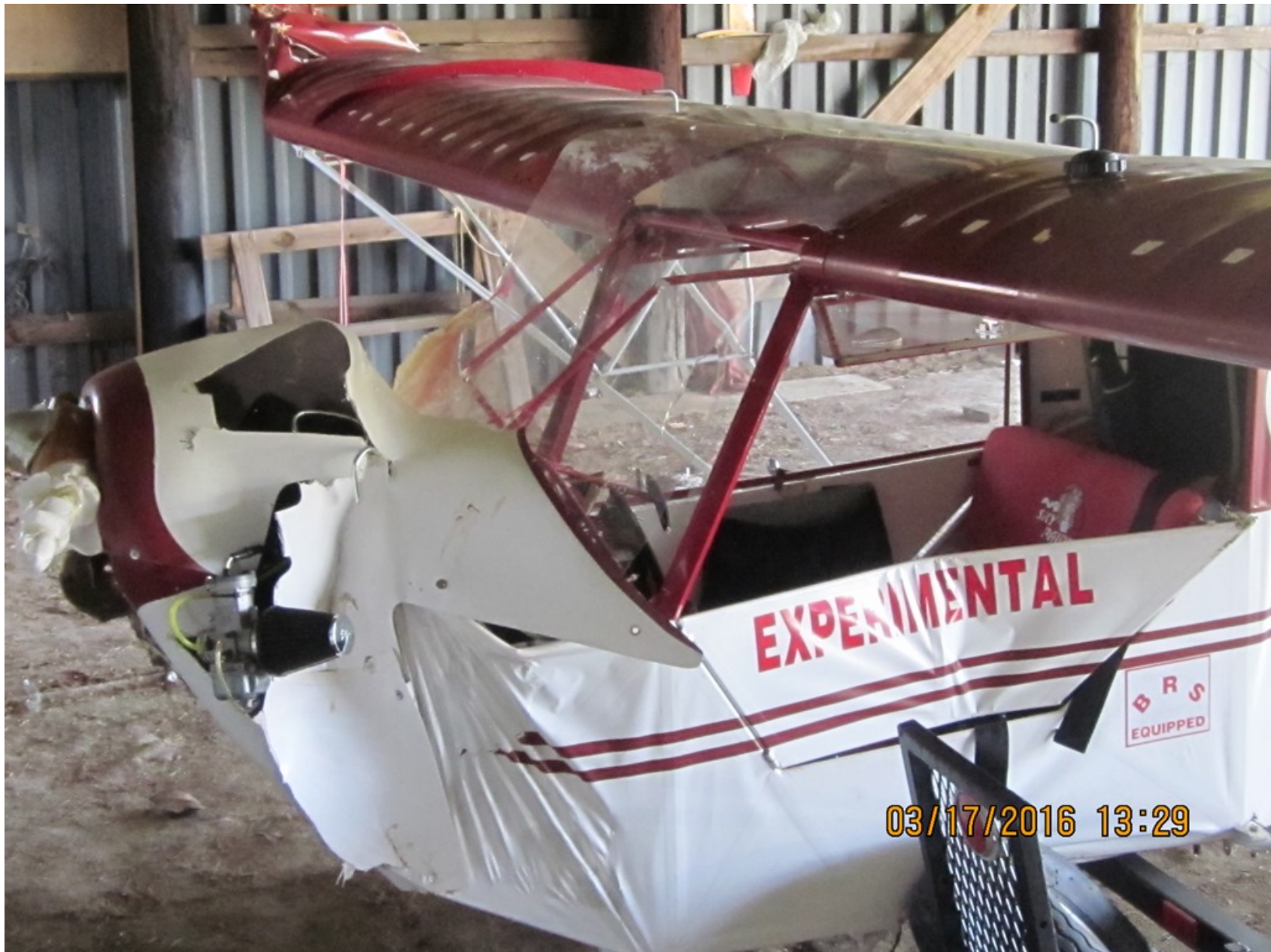
Photo 2 – View of Damage to Engine Compartment, Cockpit, and Right Wing (FAA)
