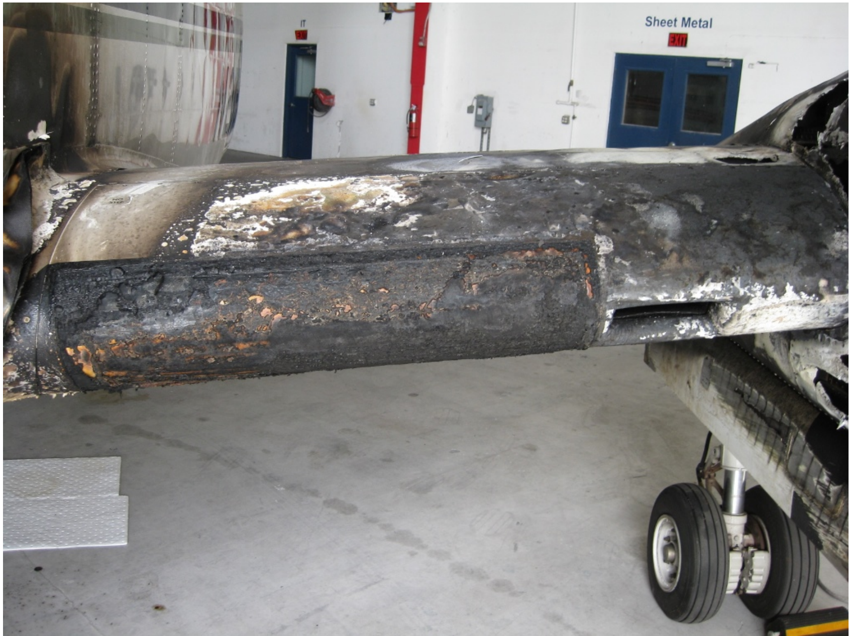
Photo 2 – View of fire damage to inboard left wing (Provided by FAA)
