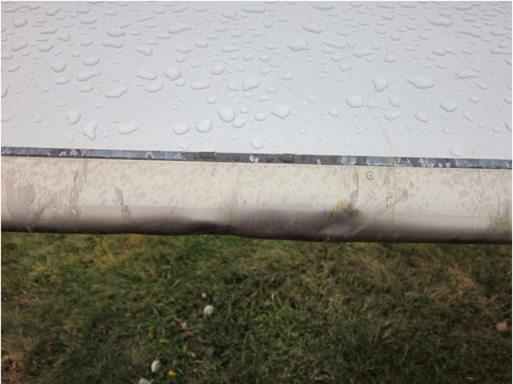
Photo 4 – Moderate Sized Dents – Courtesy of FAA
