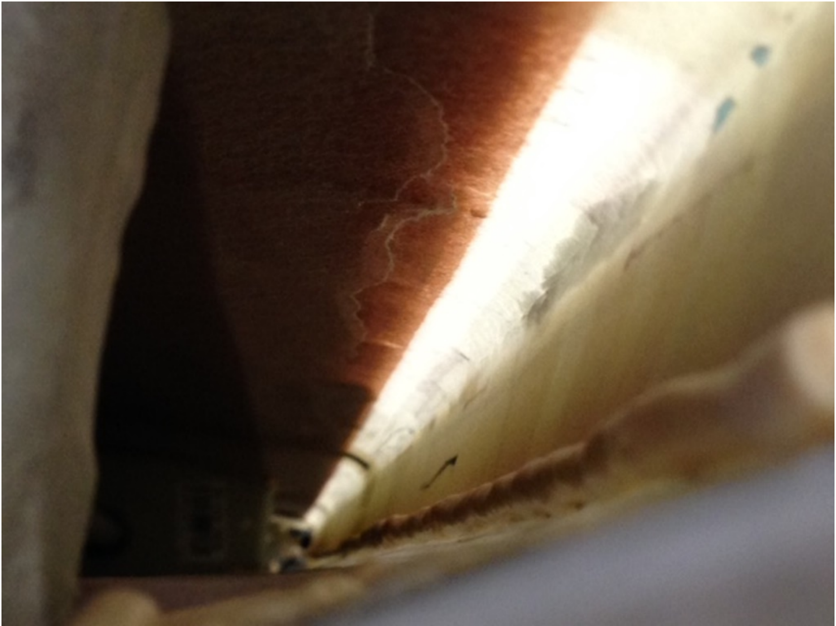
Photo 13 – Enhanced Image of interior of Damaged Wing – Courtesy of Cirrus Aircraft
