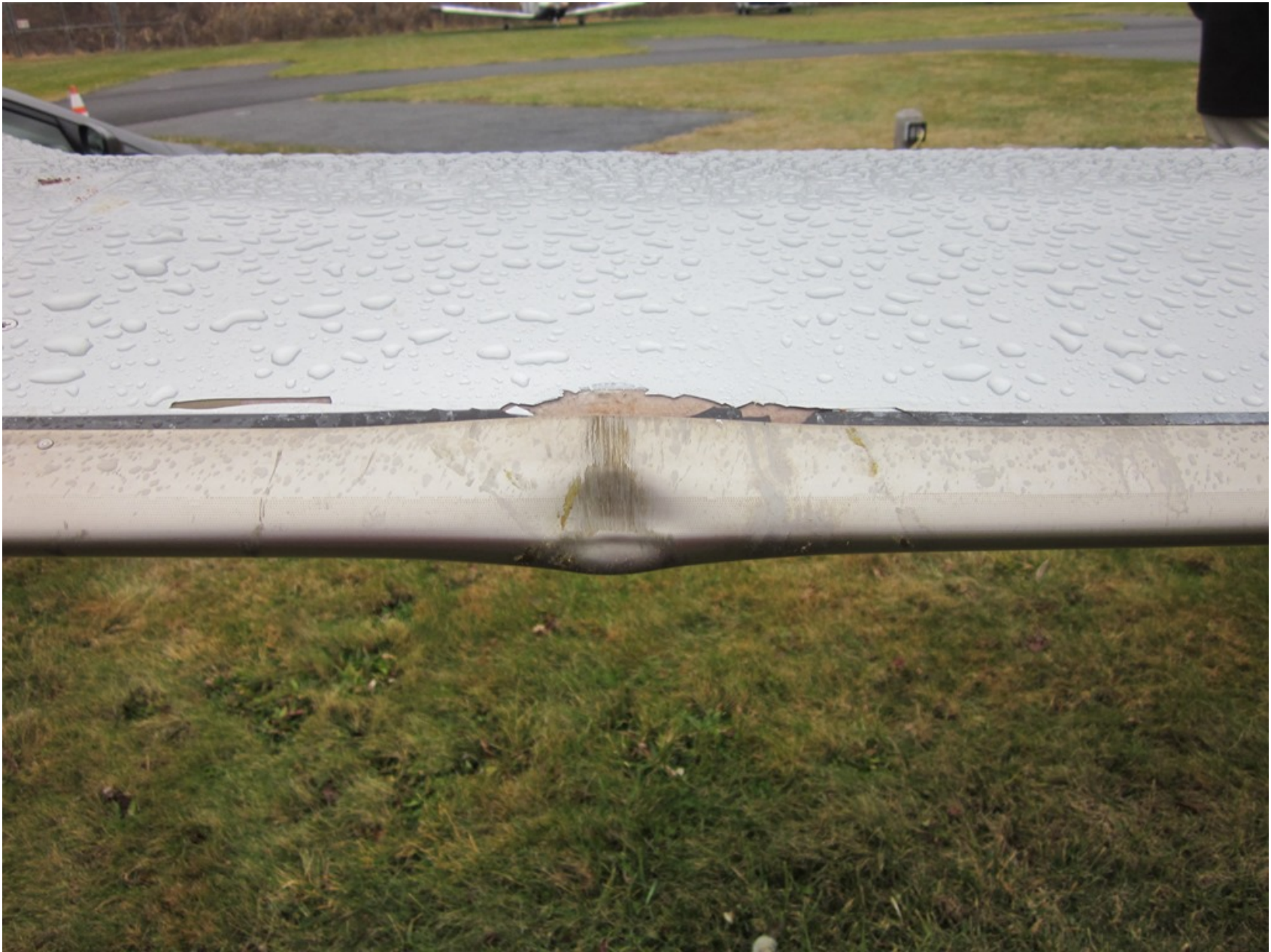
Photo 5 – Large Dent – Courtesy of FAA
