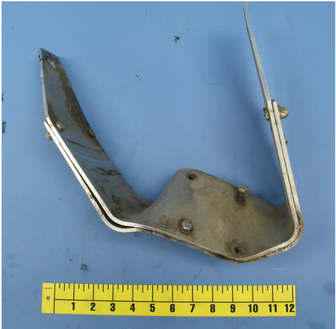
Figure 4 View showing the underside of the nose landing gear fork and doubler assembly.
