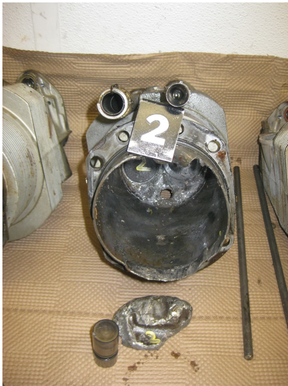
Photo 3 – No. 2 Cylinder (Photo Courtesy of FAA)
