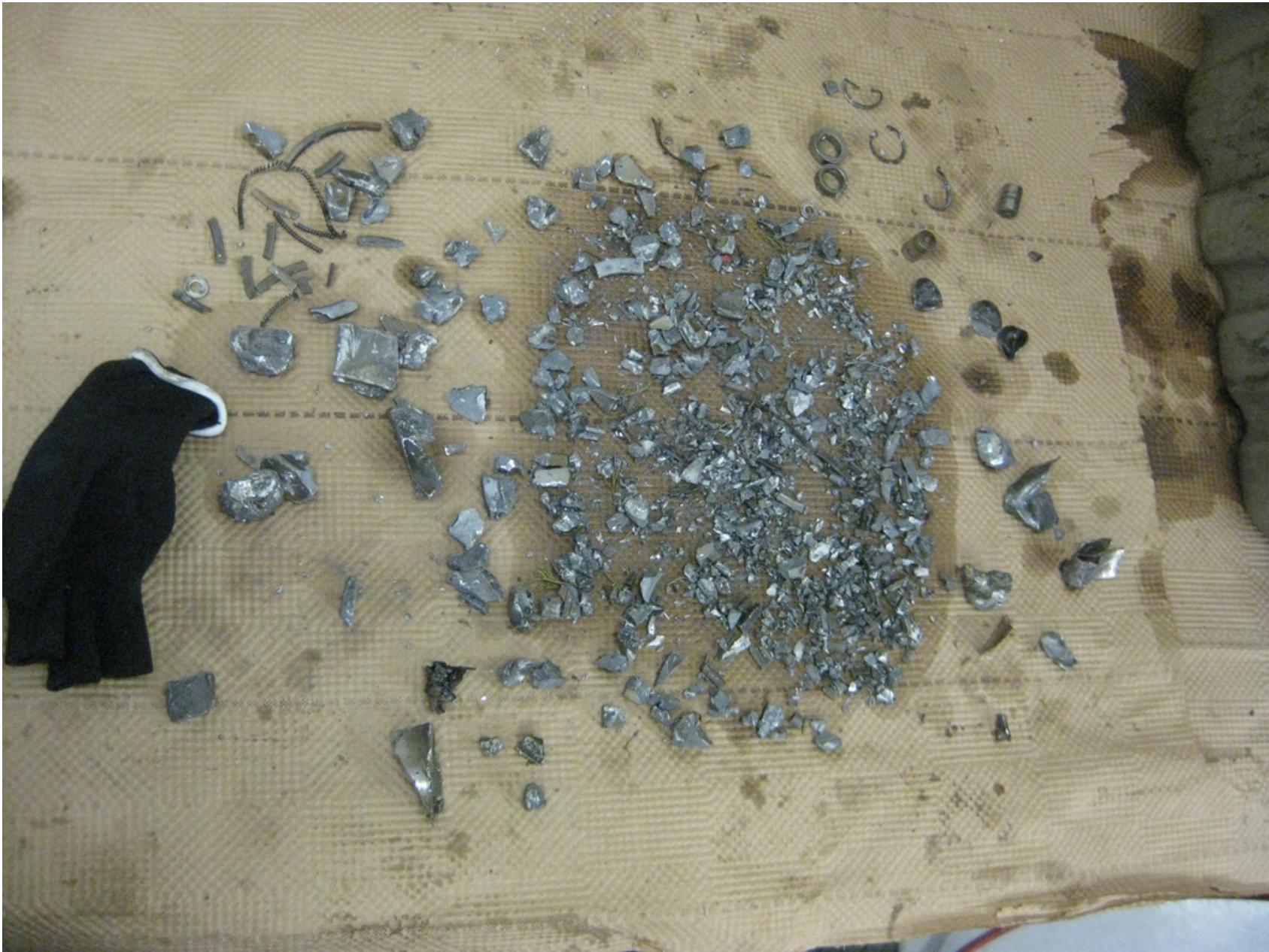
Photo 5 – No 2. Piston Fragments (Photo Courtesy of FAA)
