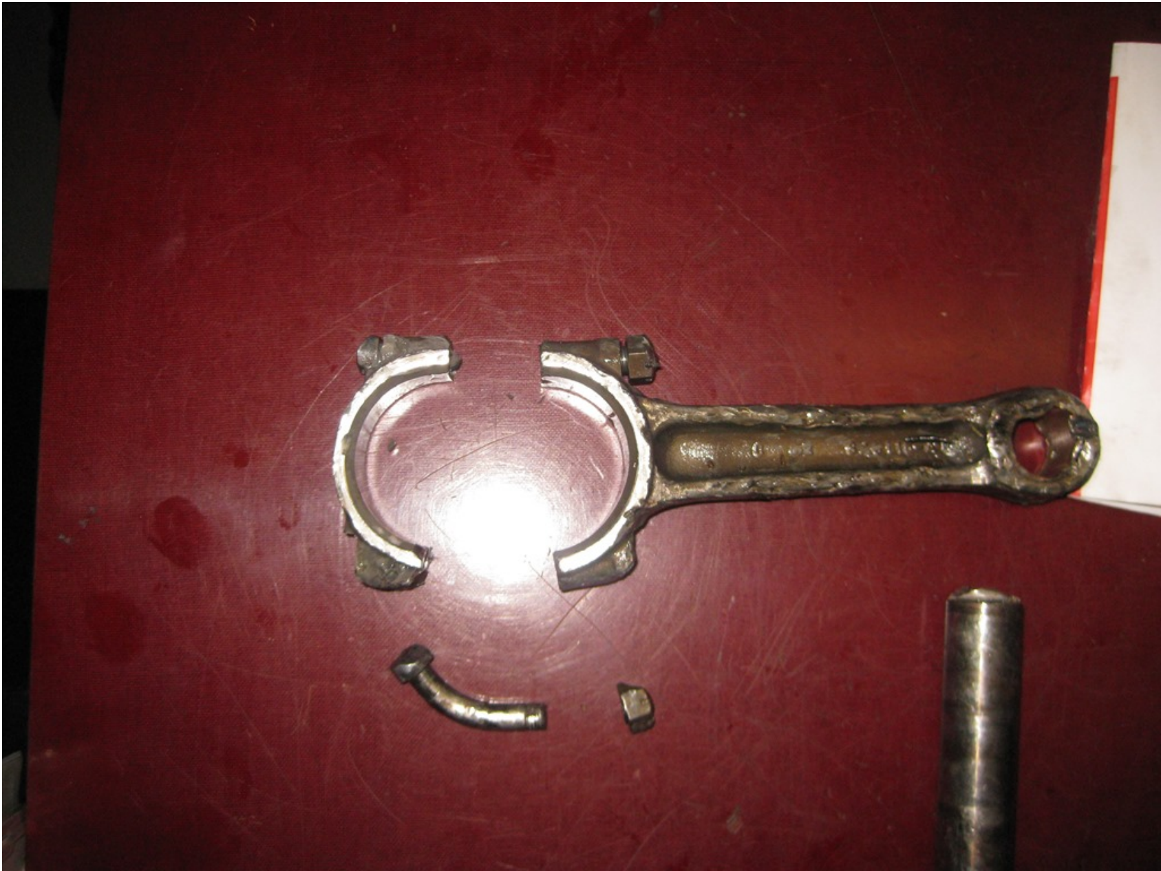
Photo 4 – No 2. Connecting Rod (Photo Courtesy of FAA)
