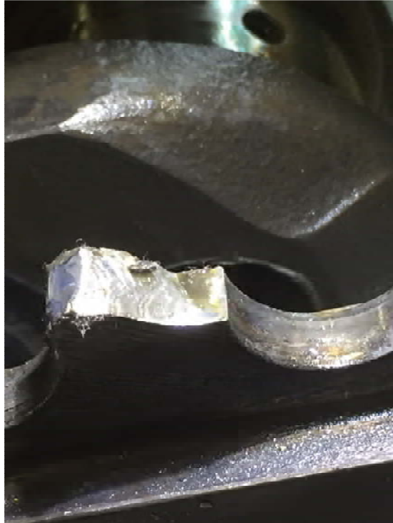
Figure 12 Fractured crankshaft aft hanger blade
