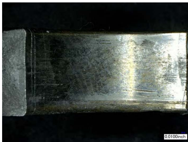
Figure 16 second fractured bushing hole
