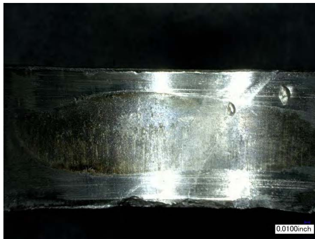
Figure 15 Bushing hole adjacent to liberated piece of hanger blade
