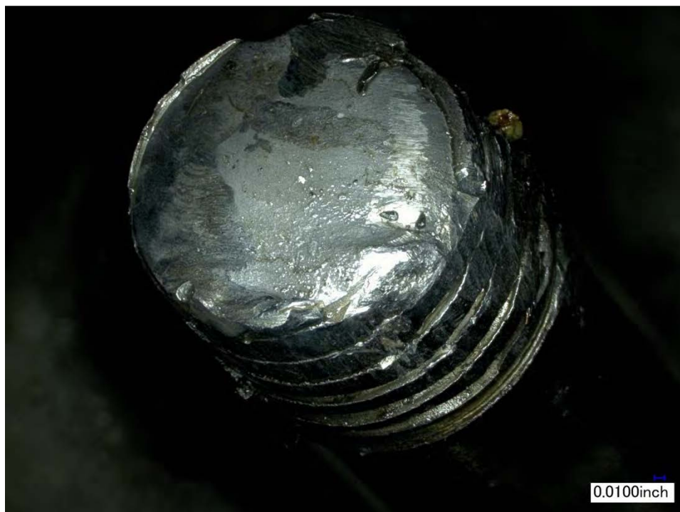
Figure 11 Rod bolt fracture surface
