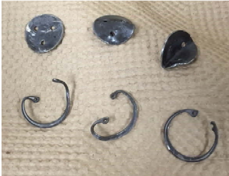
Figure 4 Liberated counterweight pin retainer plates and snap rings
