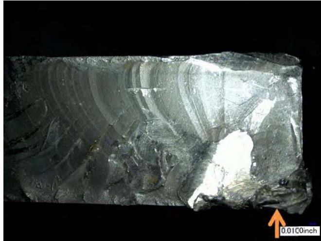
Figure 14 Liberated piece from counterweight blade shows crack growth in fatigue. Initiation area is shown by the arrow.
