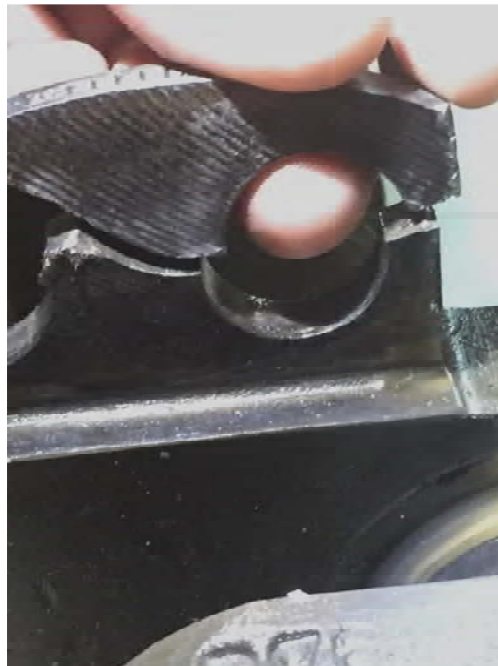
Figure 13 Aft blade with liberated piece
