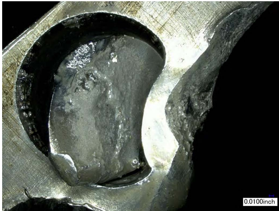
Figure 10 Bolt fracture surface
