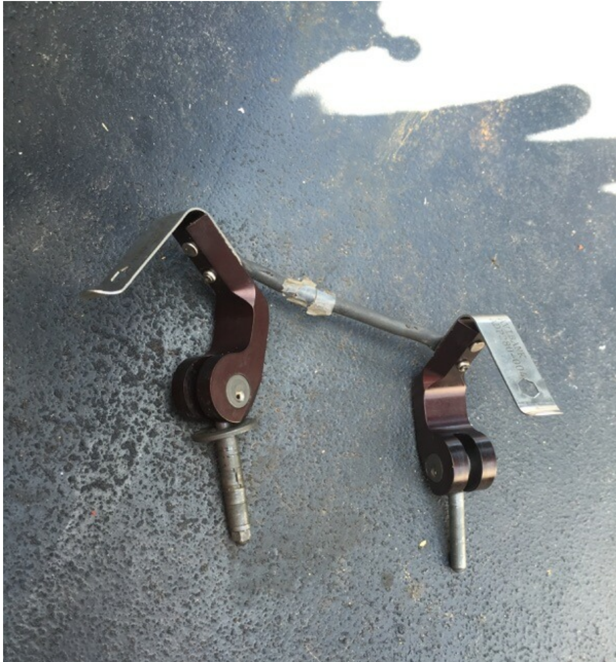
Photo 4 – View of Fractured Pin (Operator)
