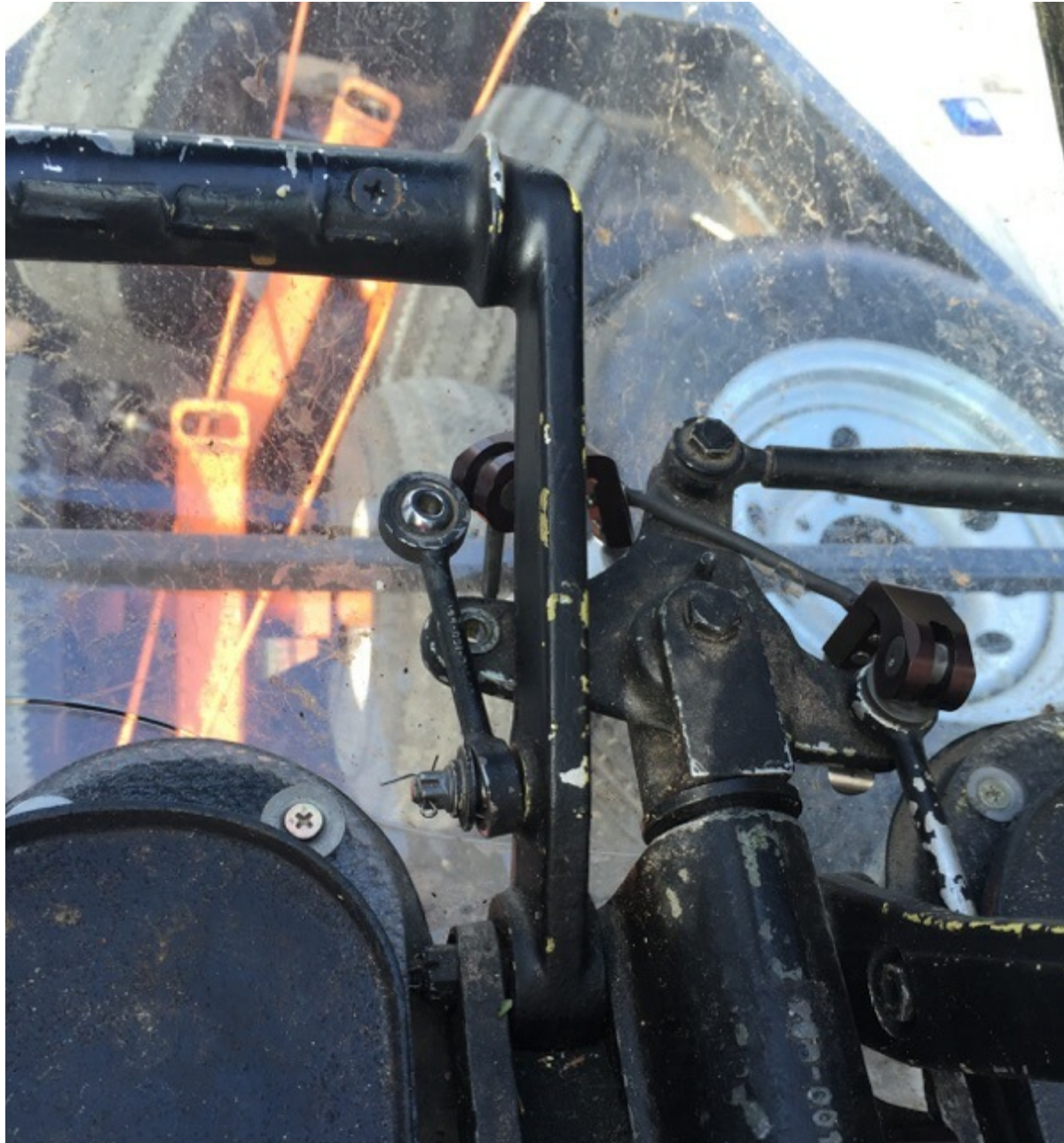
Photo 2 – View of Disconnect Left Tail Rotor Pedal Control (Operator)
