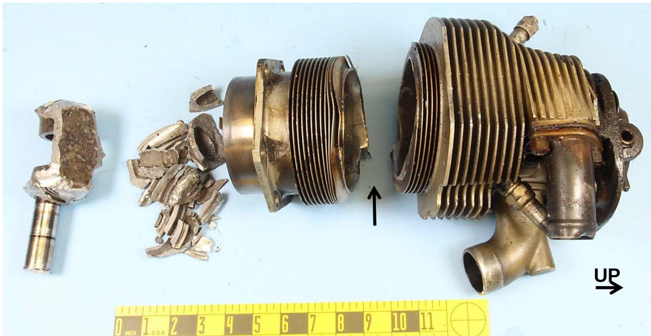
Figure 1. As-received pieces of the #4 cylinder (right side of page), fragments of the piston and piston pin that was partially inserted into the fractured piston (left side of page). The cylinder fractured in the barrel portion in the area indicated by an arrow.
