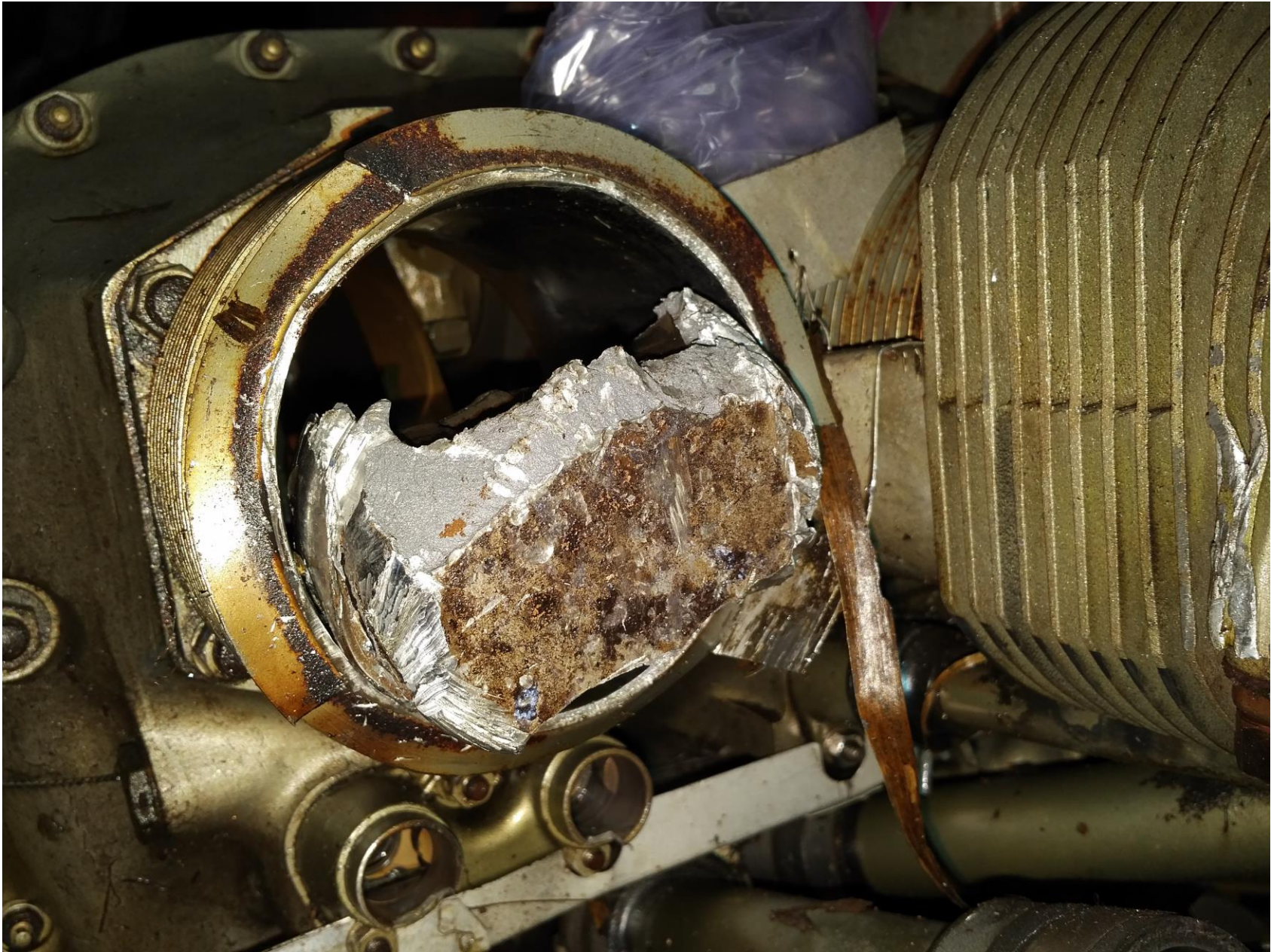
Photo 5 – View of damaged number 4 cylinder and piston.
