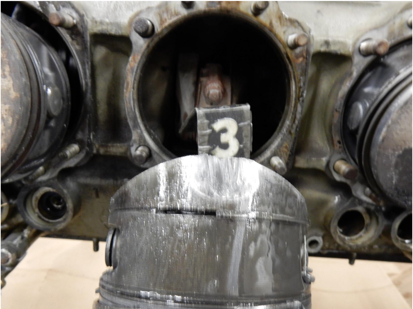
Photo 6 – View of Impact Damage to #3 Piston Skirt (FAA)
