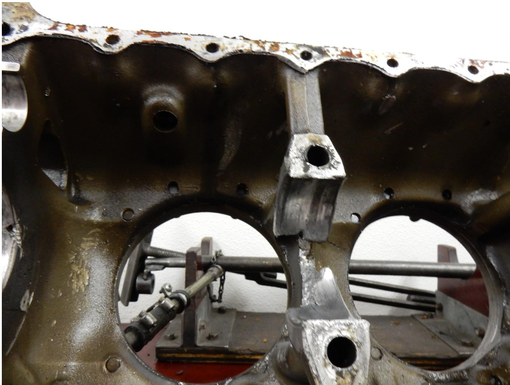
Photo 7 – View of Distressed and Fractured Main Bearing Journal (FAA)
