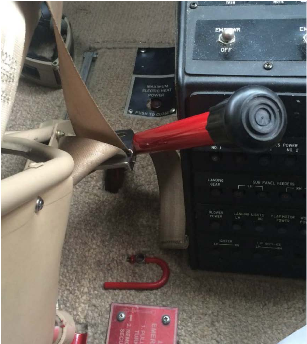
Photograph predicting posaccident position of "J" handle (Photo Courtesy of FAA).
