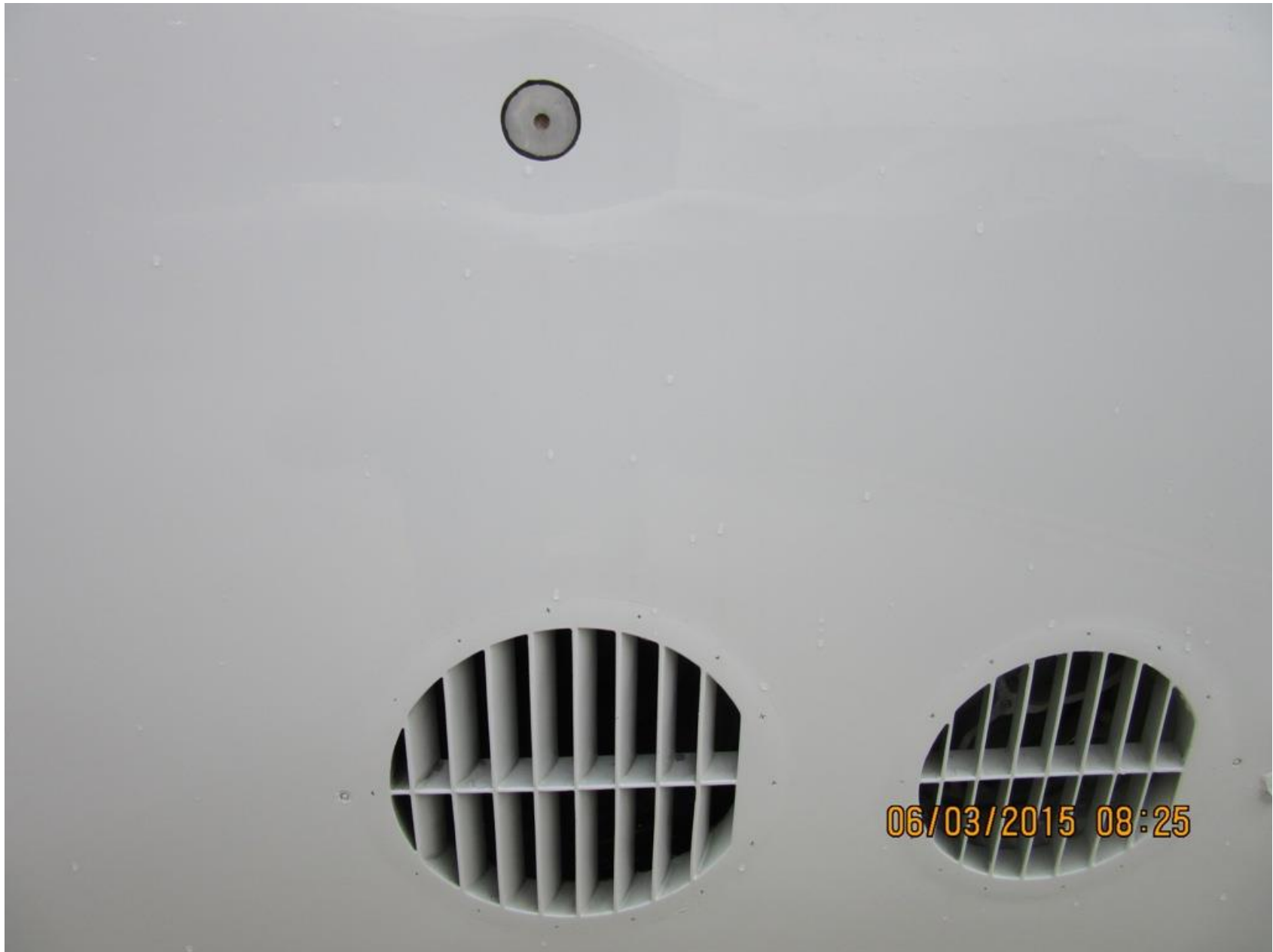
Photo 2 – Outflow Valve Safety Port
