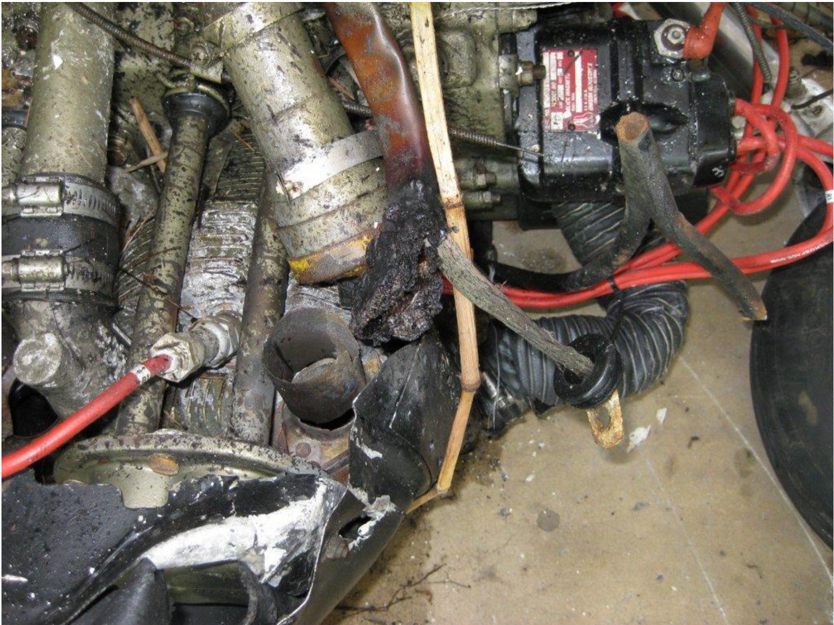
Photo 2 – Burnt Cable (Courtesy FAA)
