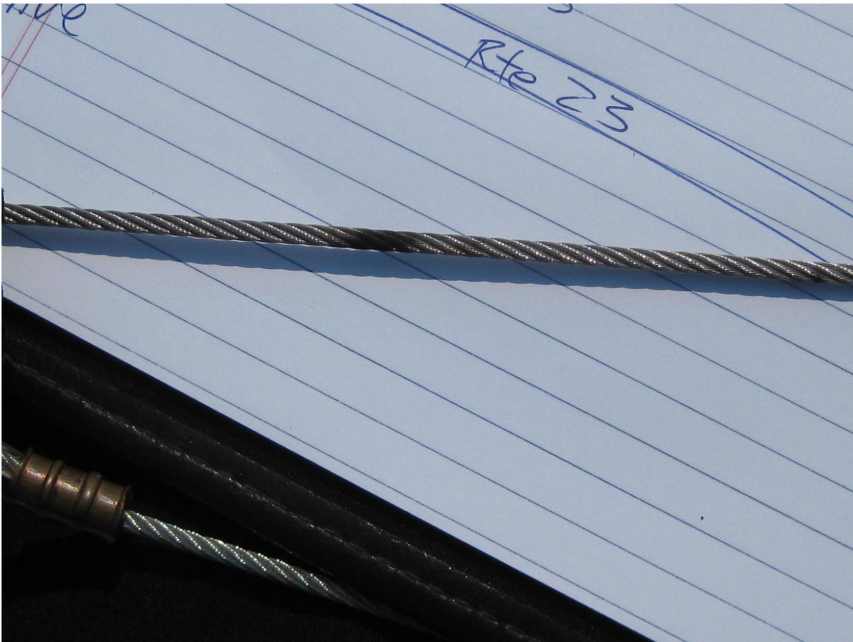
Photo 6 – Electrical Arc Burn on Basket Attach Cable (Courtesy of FAA)
