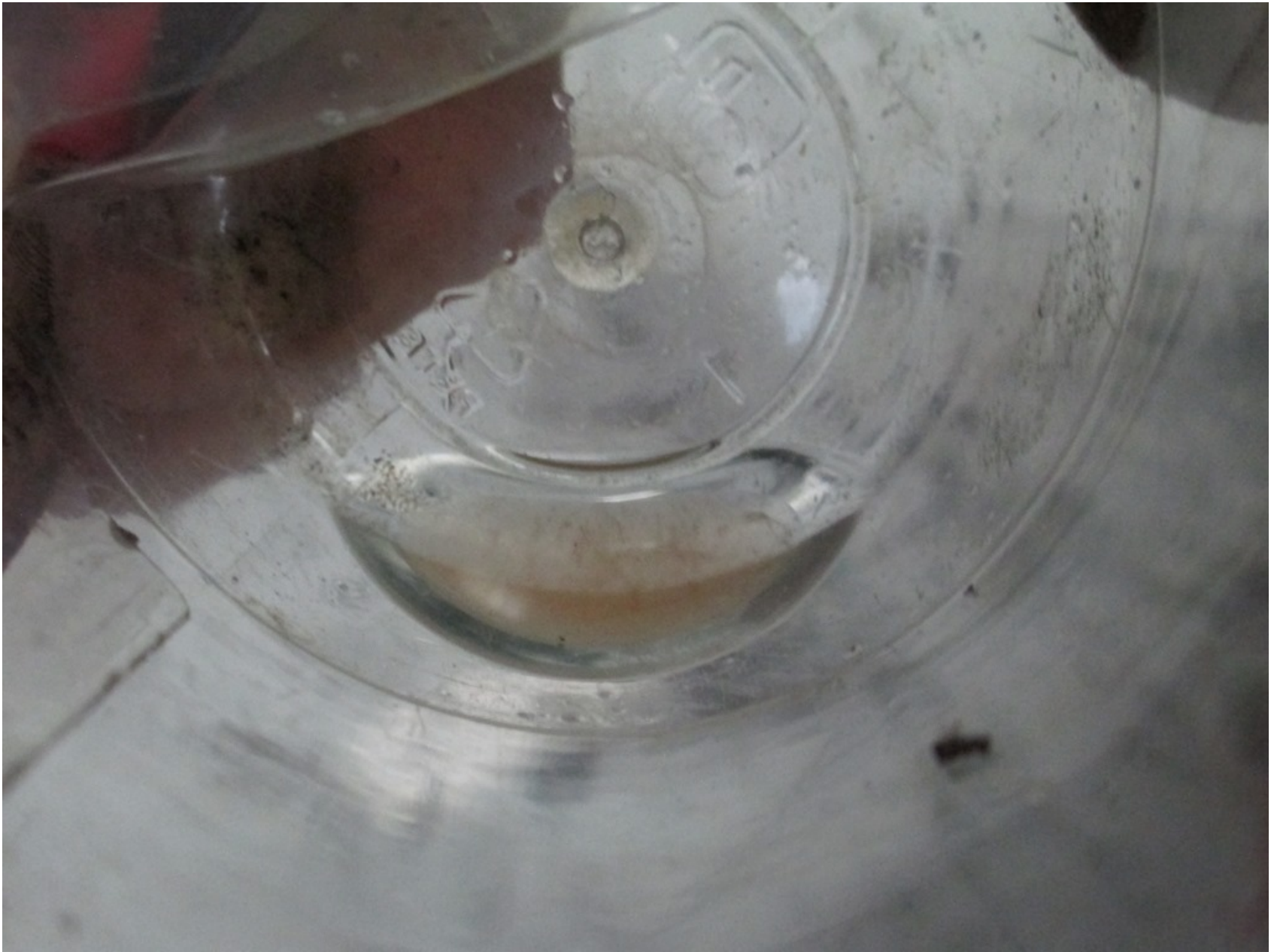
Photo 4 – Rust Colored Debris and Water Drained from Accelerator Pump
