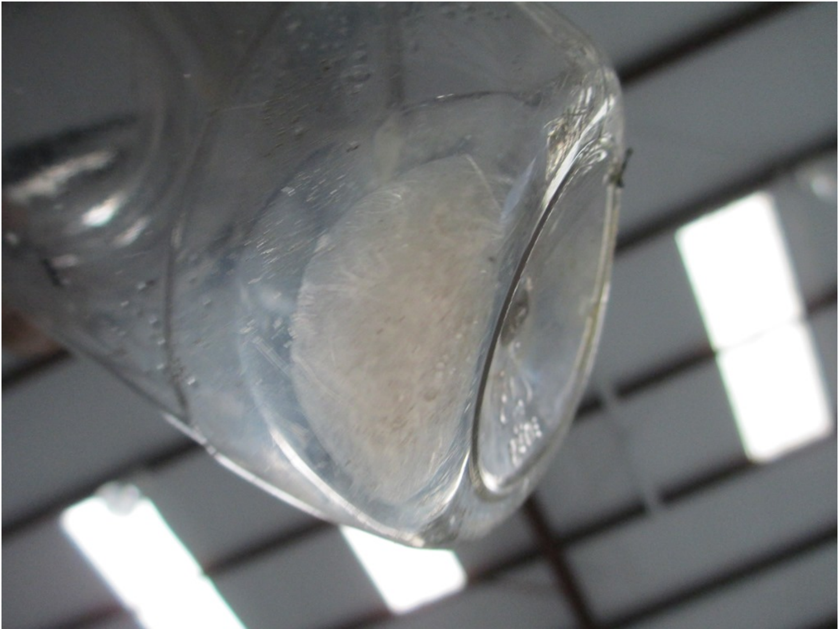
Photo 3 – Rust-Colored Debris and Water Drained from Accelerator Pump
