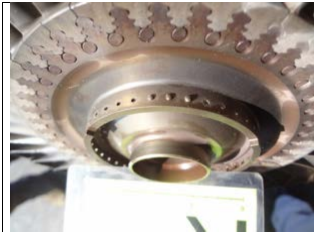
Photo 40: Two Parallel Minor Score Marks on Inner Section
