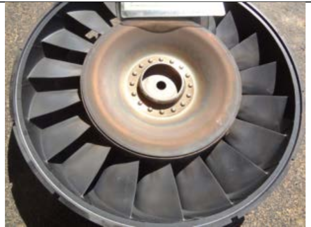
Photo 41: Power Turbine Vane Baffle
