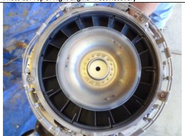
Photo 31: Power Turbine Baffle
