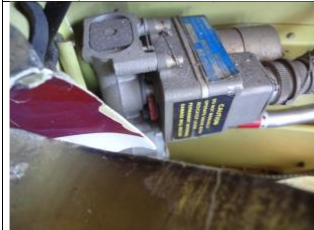
Photo 38: Fuel Shutoff Valve as Found
