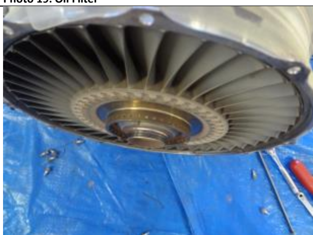
Photo 21: Power Turbine Disc with Rotational Score Marks
