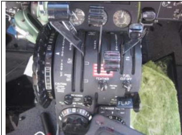
Photo 10: Power Lever Quadrant as Viewed on Scene (Courtesy of FAA)
