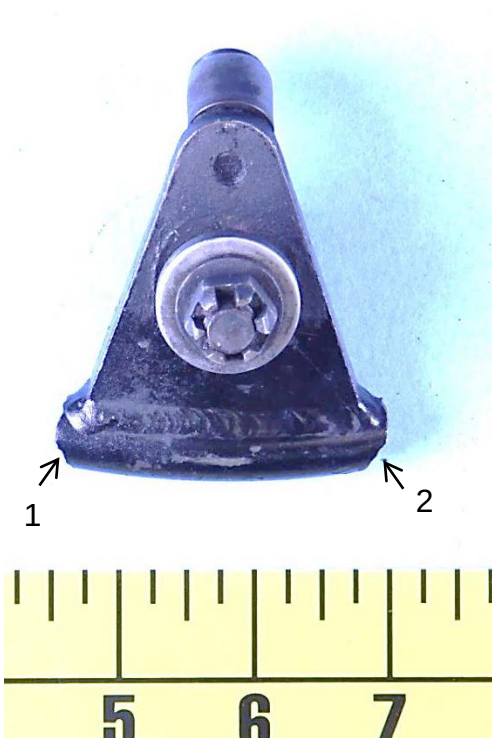
Figure 1. Photograph of the as-received engine mount that fractured at two areas indicated by arrows "1" and "2".
