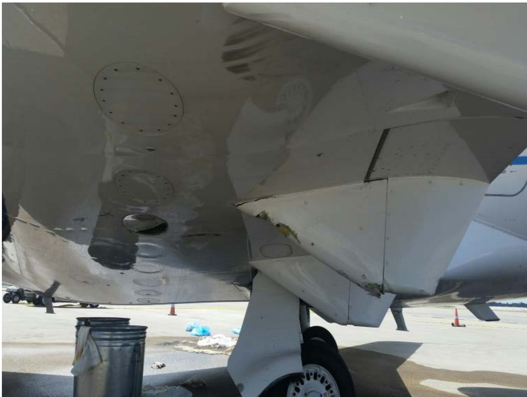
Photo 3 – Bottom of left wing damage (Courtesy of McLarens Claim Serv.)
