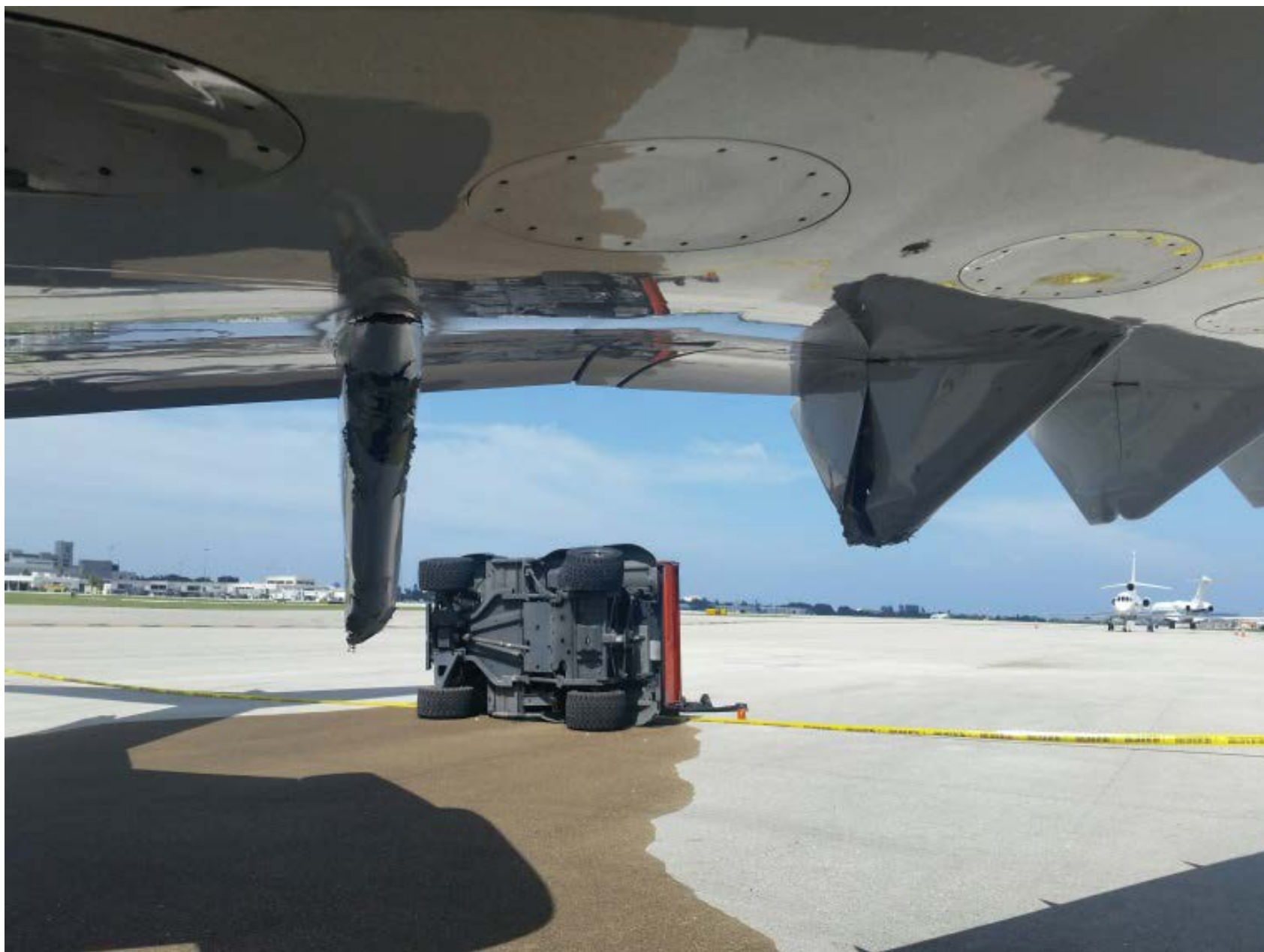
Photo 4 – Damaged left wing and ATV that was struck (Courtesy of McLarens Claim Serv.)
