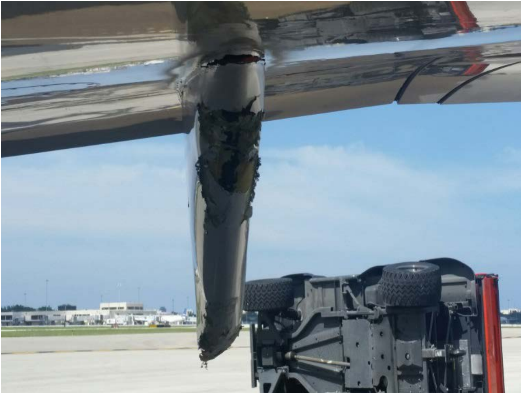
Photo 1 – Damaged left wing (courtesy of McLarens claim Serv.)
