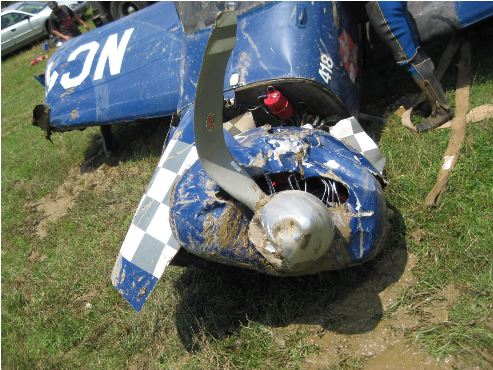
Photo 4 – Airplane Engine and Propeller Damage (Courtesy of FAA)
