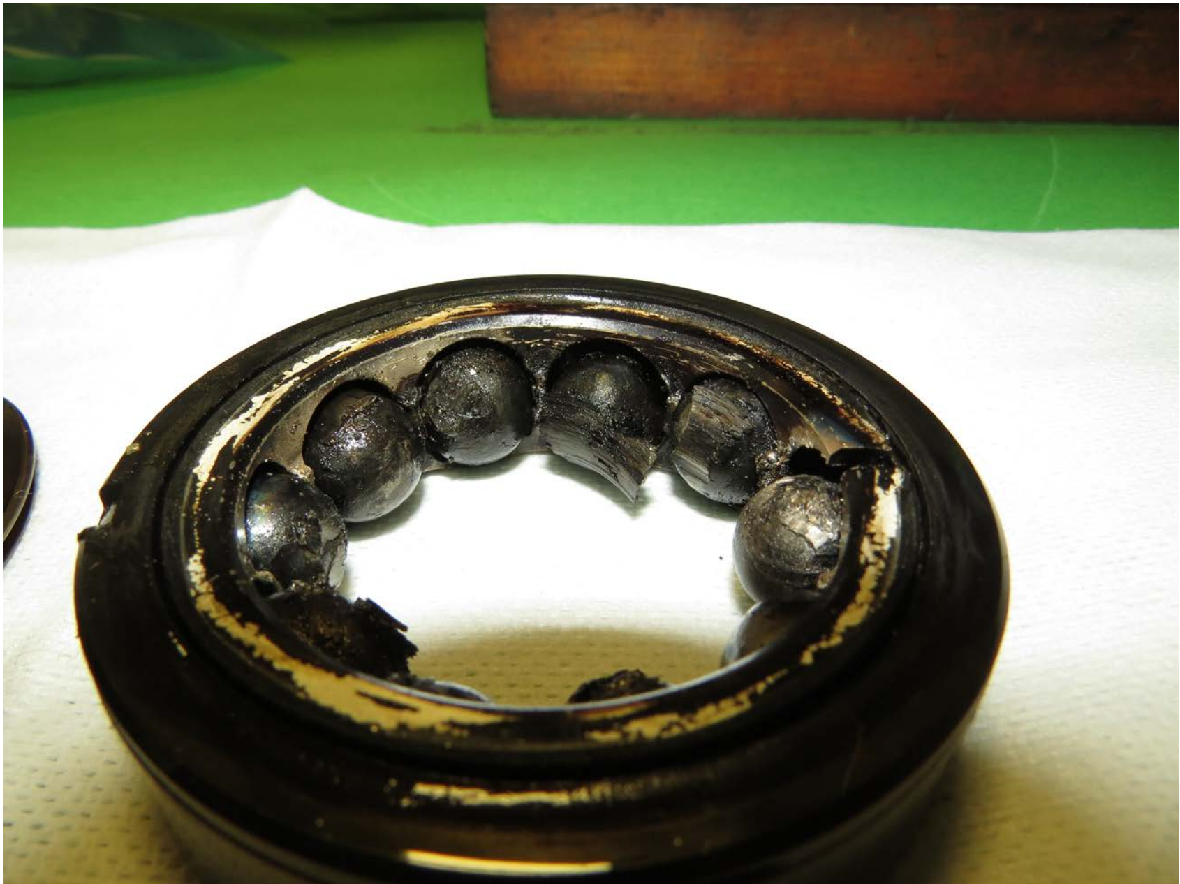
Photo 5 – Damaged Number 2 Bearing, Removed (Photo Courtesy of FAA)
