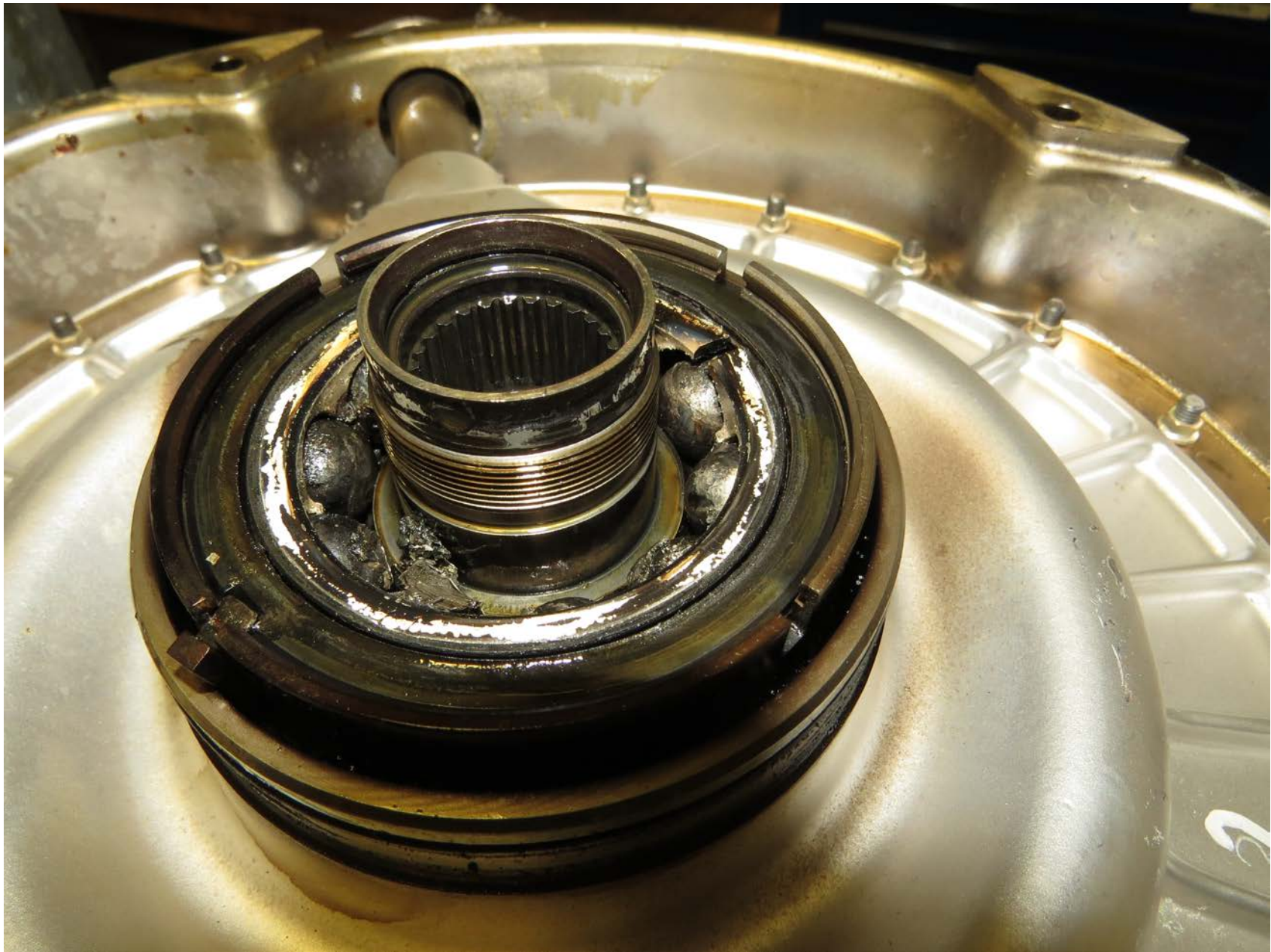
Photo 4 – Damaged Number 2 Bearing (Photo Courtesy of FAA)
