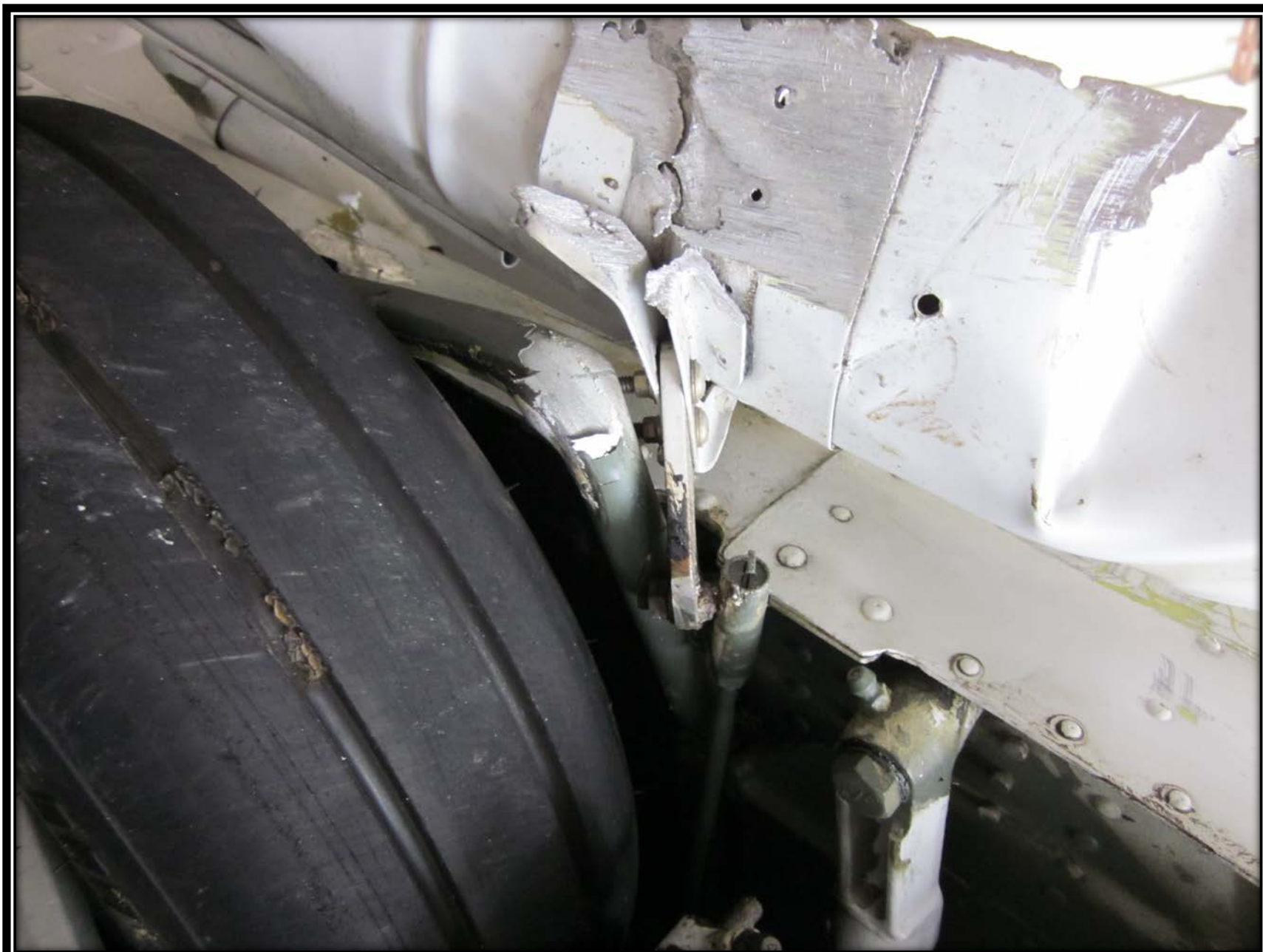
Photo 8 – Nose Gear Damage (Photo Courtesy of FAA)
