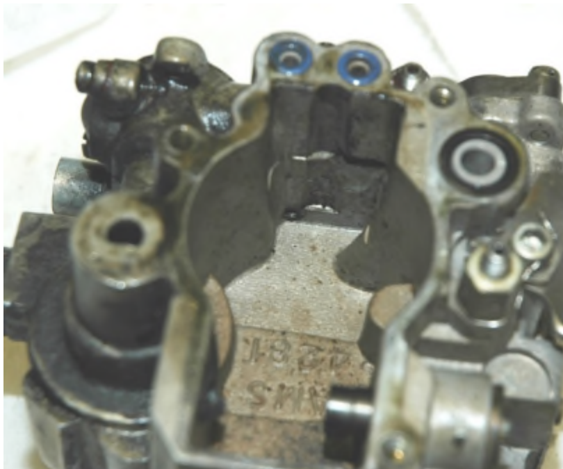
Photo No.28 Fuel control unit flow body.
