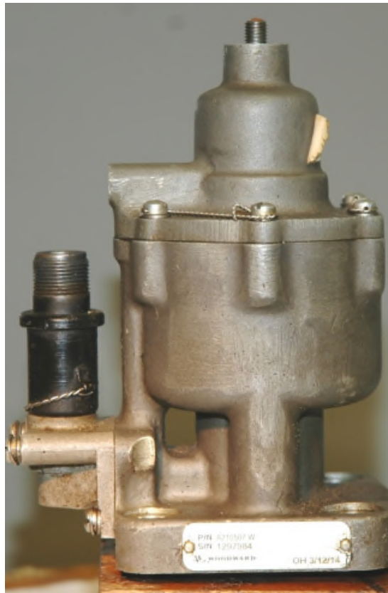
Photo No. 34 Propeller overspeed governor, as received.
