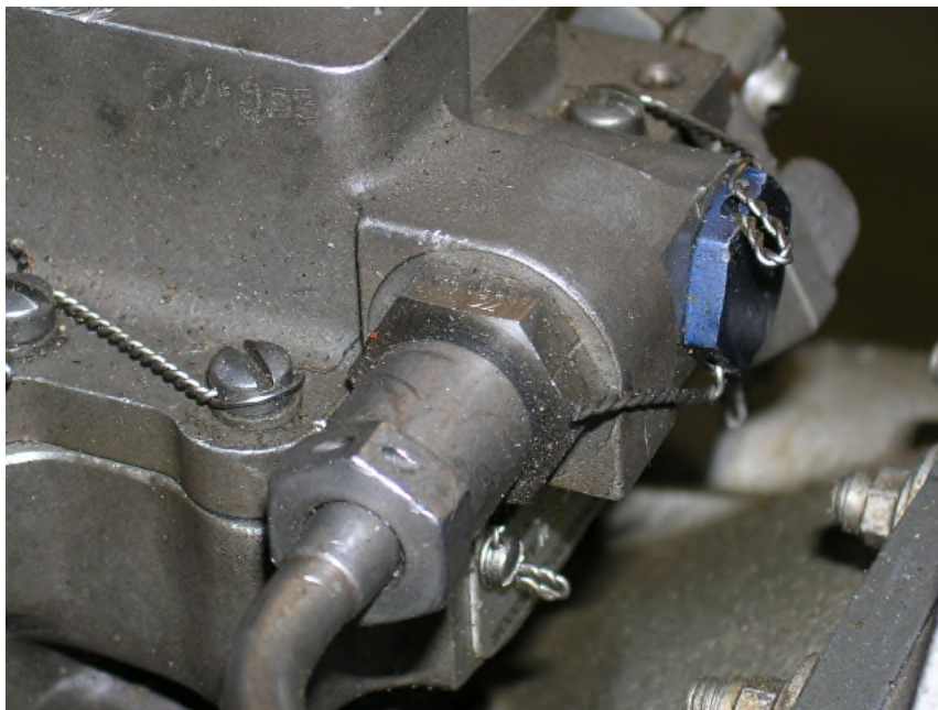
Photo No. 7 Propeller governor Py fitting, detail.
