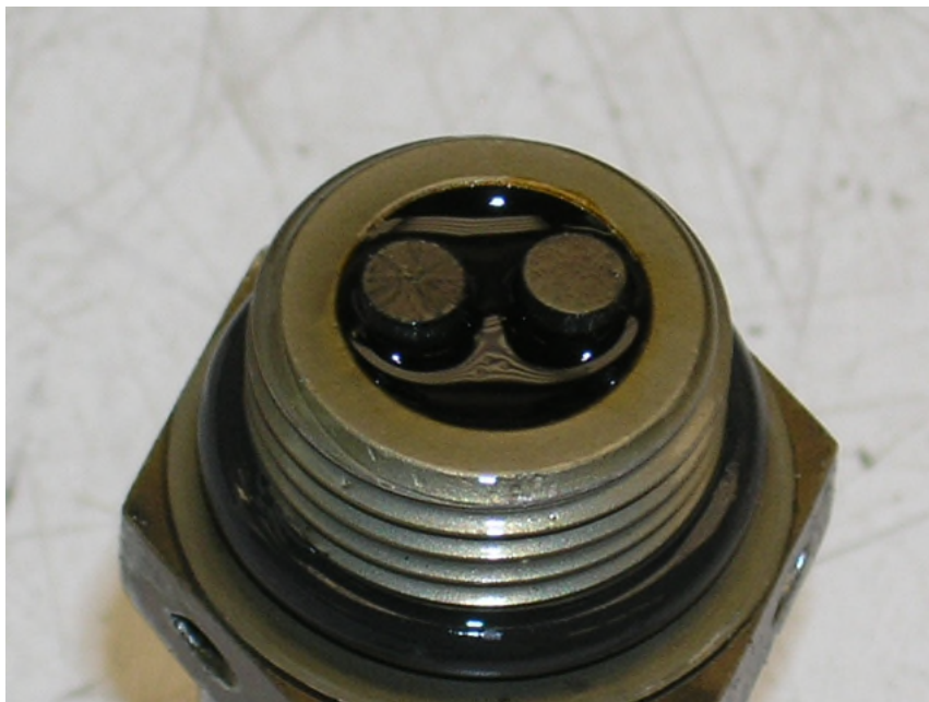
Photo No. 9 Reduction gearbox chip detector.
