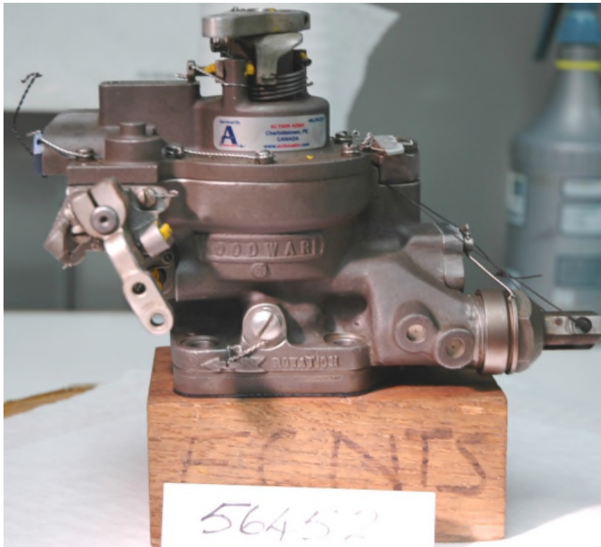
Photo No. 30 Propeller governor as removed.
