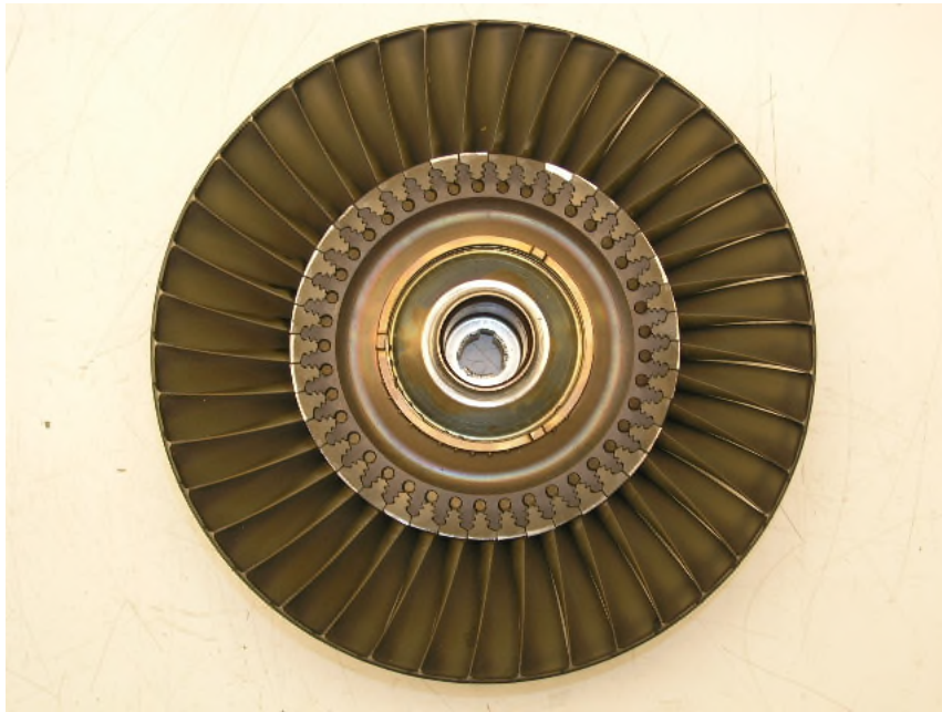
Photo No. 19 Power turbine, upstream side.
