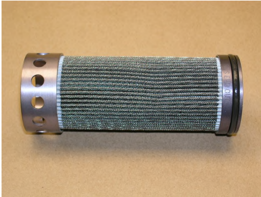
Photo No. 10 Oil filter.
