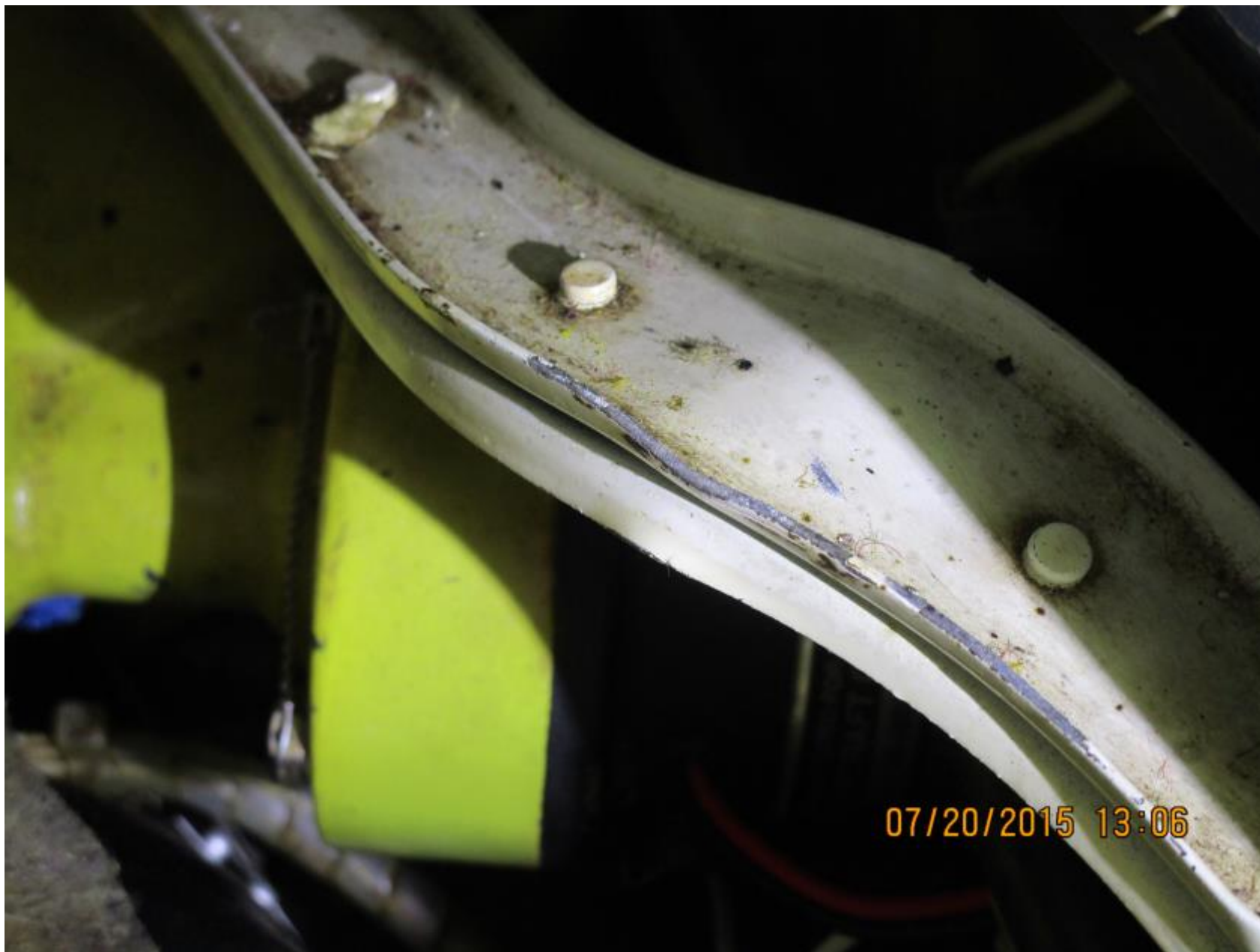
Photo 9 - Right Main Gear Extension Rod at Gearbox (Courtesy of the FAA)
