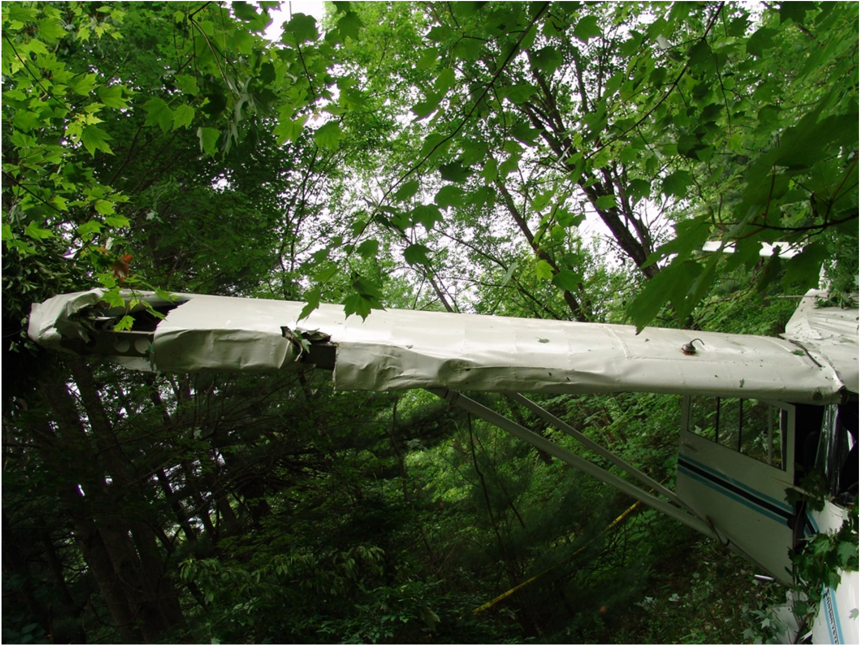
Photo 4 – Right Wing Damage (FAA Photo)
