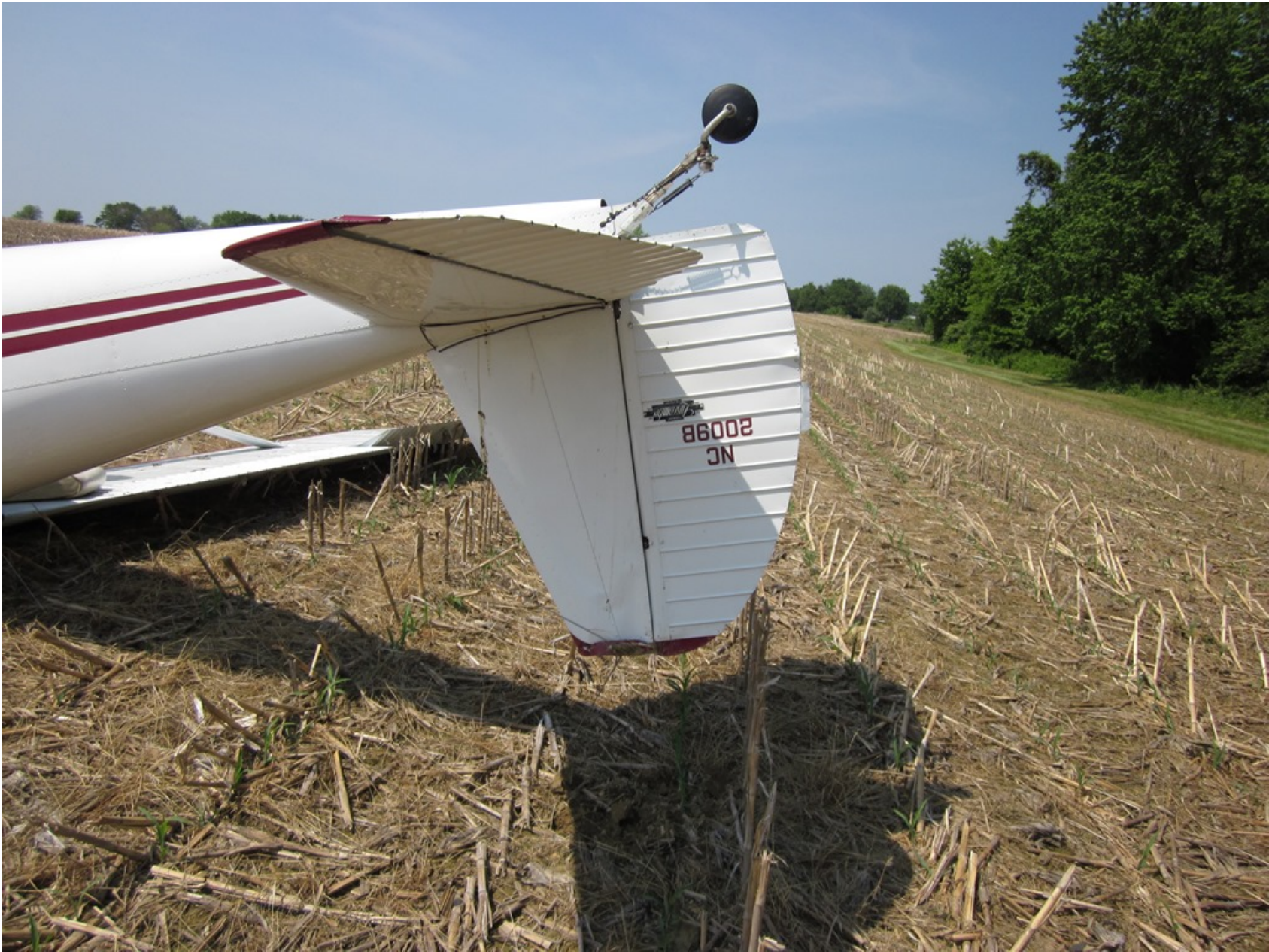
Photo 3 - View of Vertical Stabilizer Damage (Courtesy of FAA)
