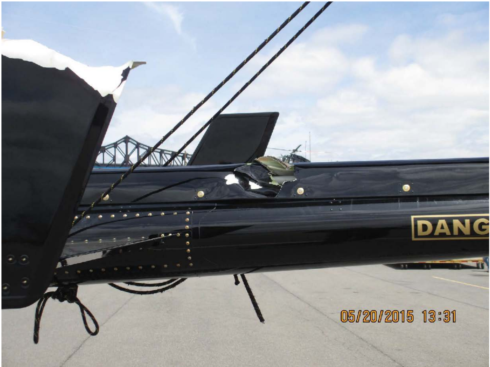
Photo 2 – Tail Boom Damage (Photo Courtesy of FAA)
