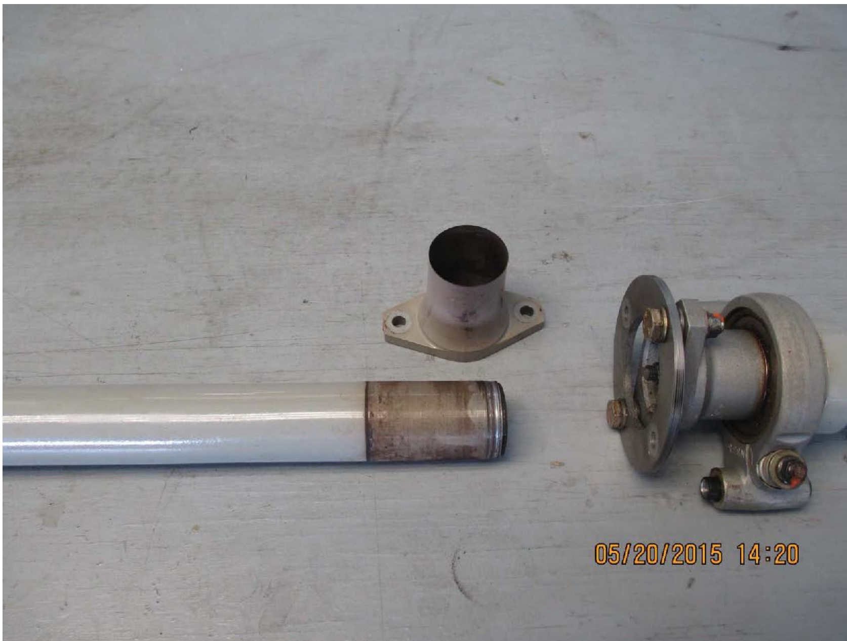
Photo 3 – Section of Tail Rotor Driveshaft
