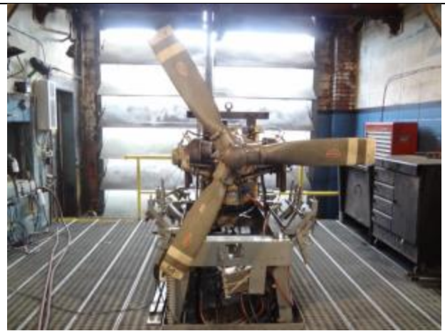
Photo 19: Front Side of Engine on Test Stand
