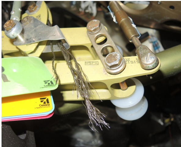
Photo 2: Right Aileron cable as found at Control Stick Connection (Courtesy of Textron)
