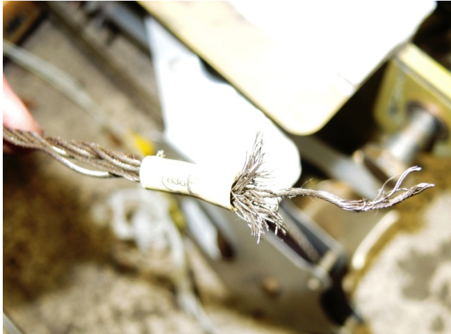
Photo 1: Right Aileron Cable as Found (Courtesy of Textron)
