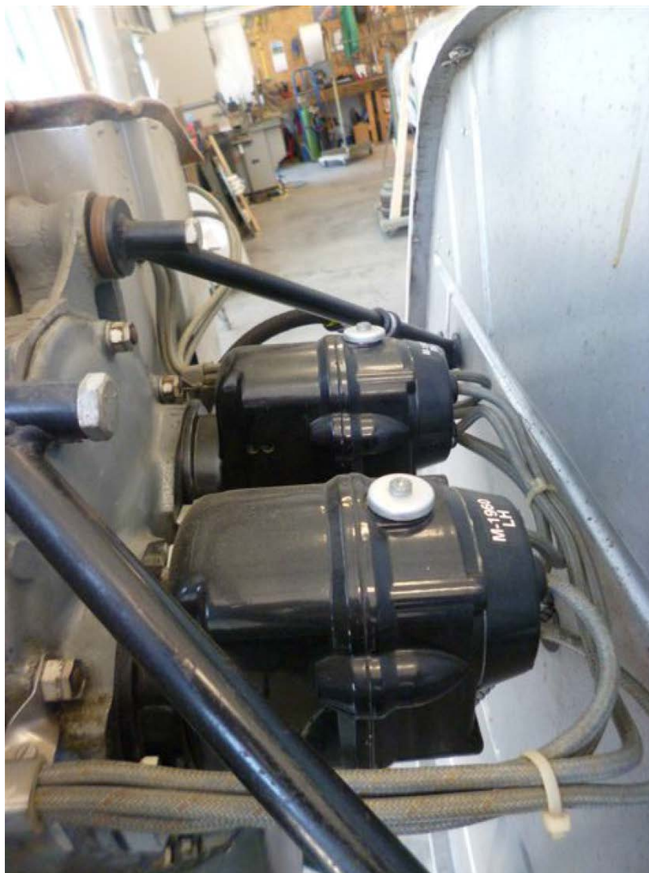
Photo 6 – Magnetos – Courtesy of AIG Aerospace
