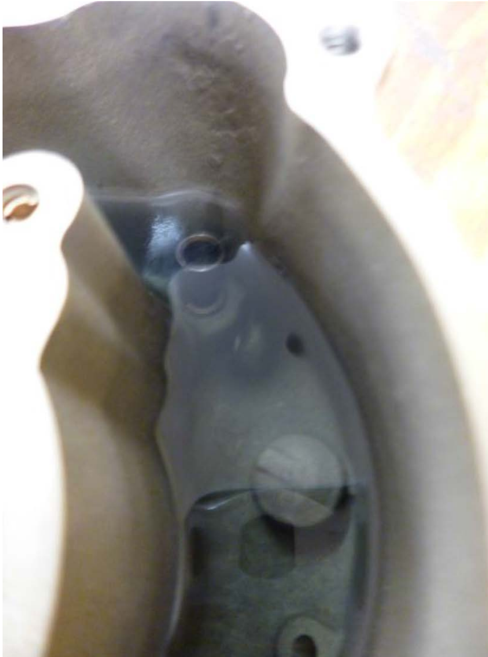
Photo 12 – Close Up Photo of Fuel in Float Bowl – Courtesy of AIG Aerospace
