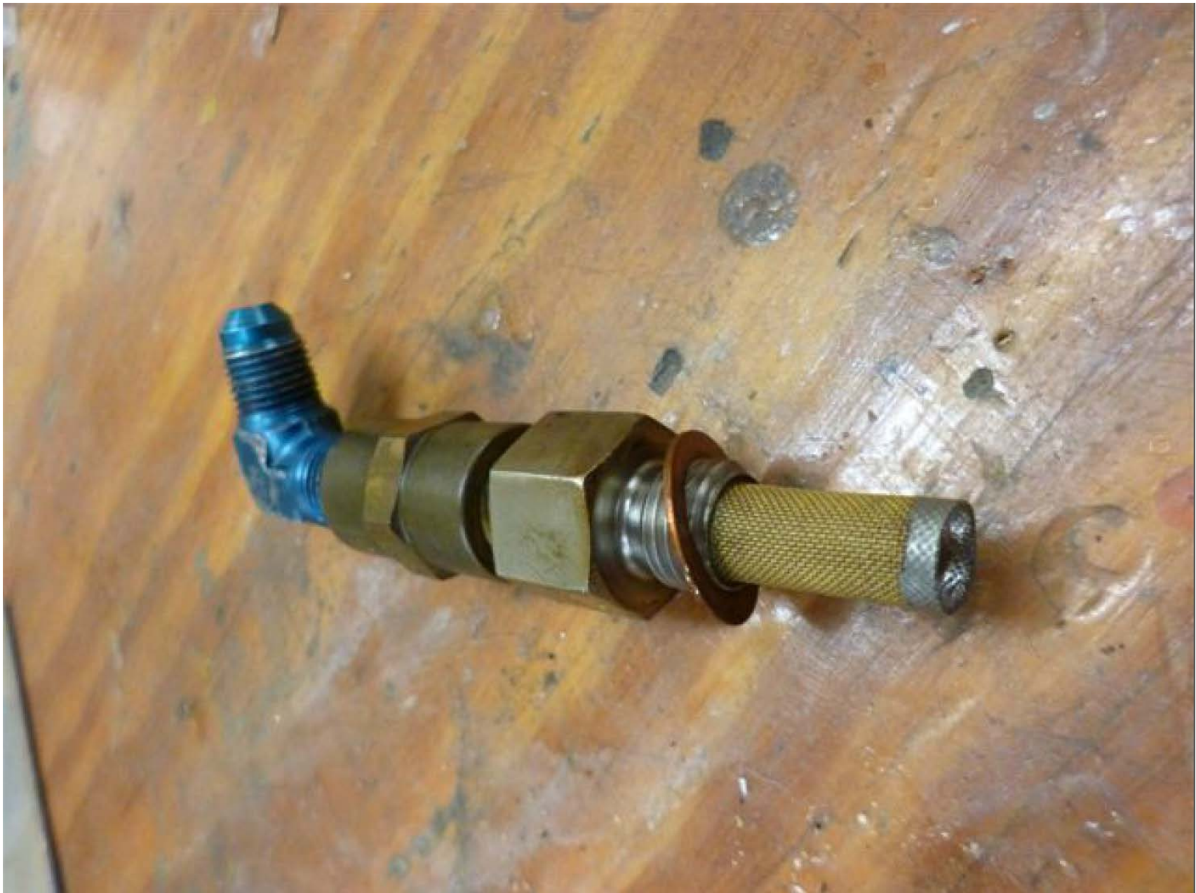
Photo 8 – Fuel Screen – Courtesy of AIG Aerospace
