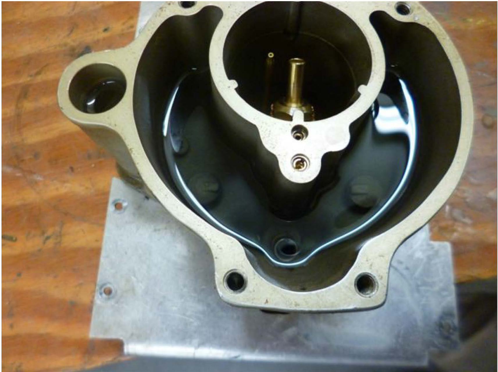
Photo 11 – Carburetor Float Bowl – Courtesy of AIG Aerospace
