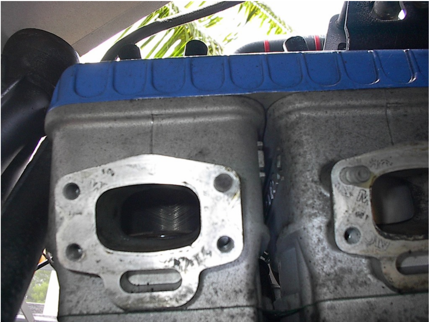
Photo 4 - Photo 3 - Digital Photograph Provided by Owner. View Depicting the Piston Sides of the Rear Cylinder. No Scuffing or Scoring was Noted on the Piston. Hone marks are Visible on the Forward Cylinder Walls
