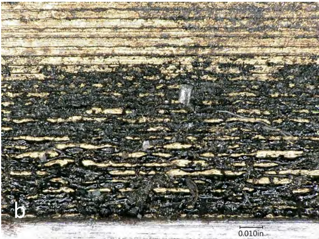
Figure 9 Close views of the number 5580 Lamiflex bearing outside diameter surface.
