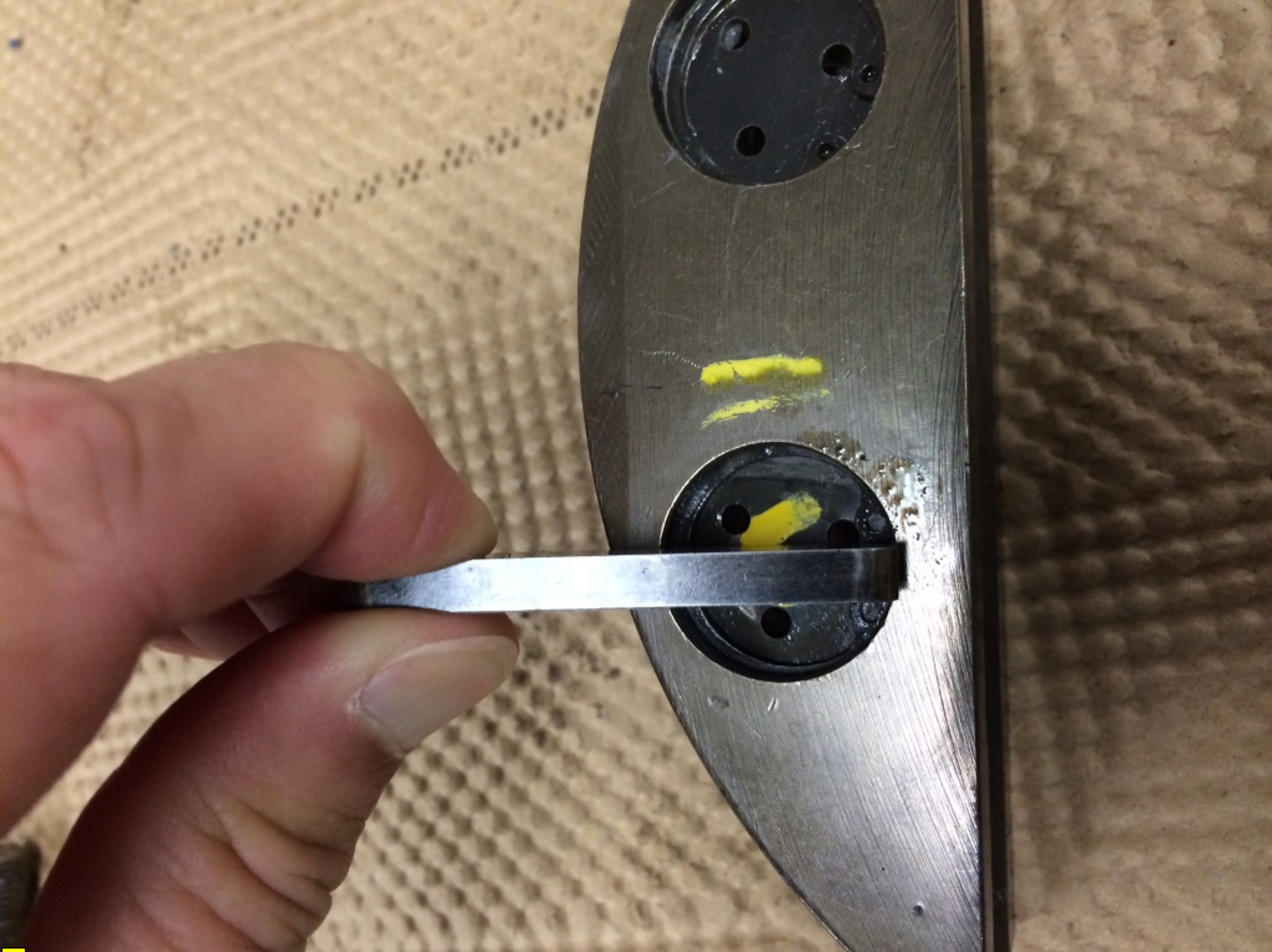
Photo 7 – Snap Rings on Rear Upper Counterweight When Cleaned And Gauge Did Fit
